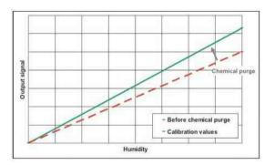
The purge function briefly heats the sensor in order to remove any volatile contaminants from the polymer.
