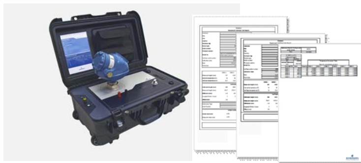
Figure 4. NIST-Traceable Verification Box
