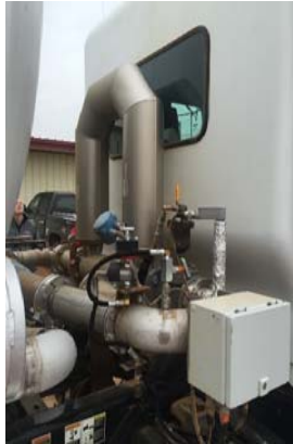
Figure 6. Trailer Mounted Coriolis System
