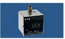
Continuous Cleaning Valve (CCV) is the standard configuration where the cleaning disc continuously cycles, driven by shop airflow. Purge is controlled by a manual valve or push-button.
