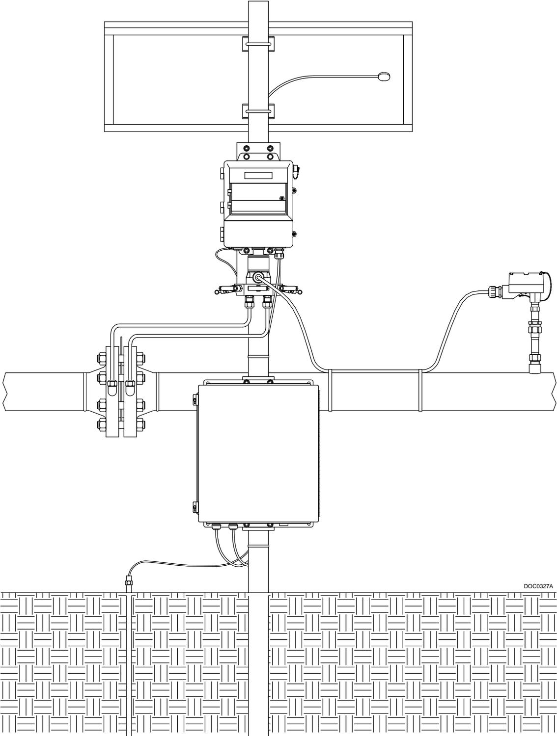
Figure 5-3. Installation with Pipestand Mounted Battery Enclosure (FloBoss 407 Shown)
