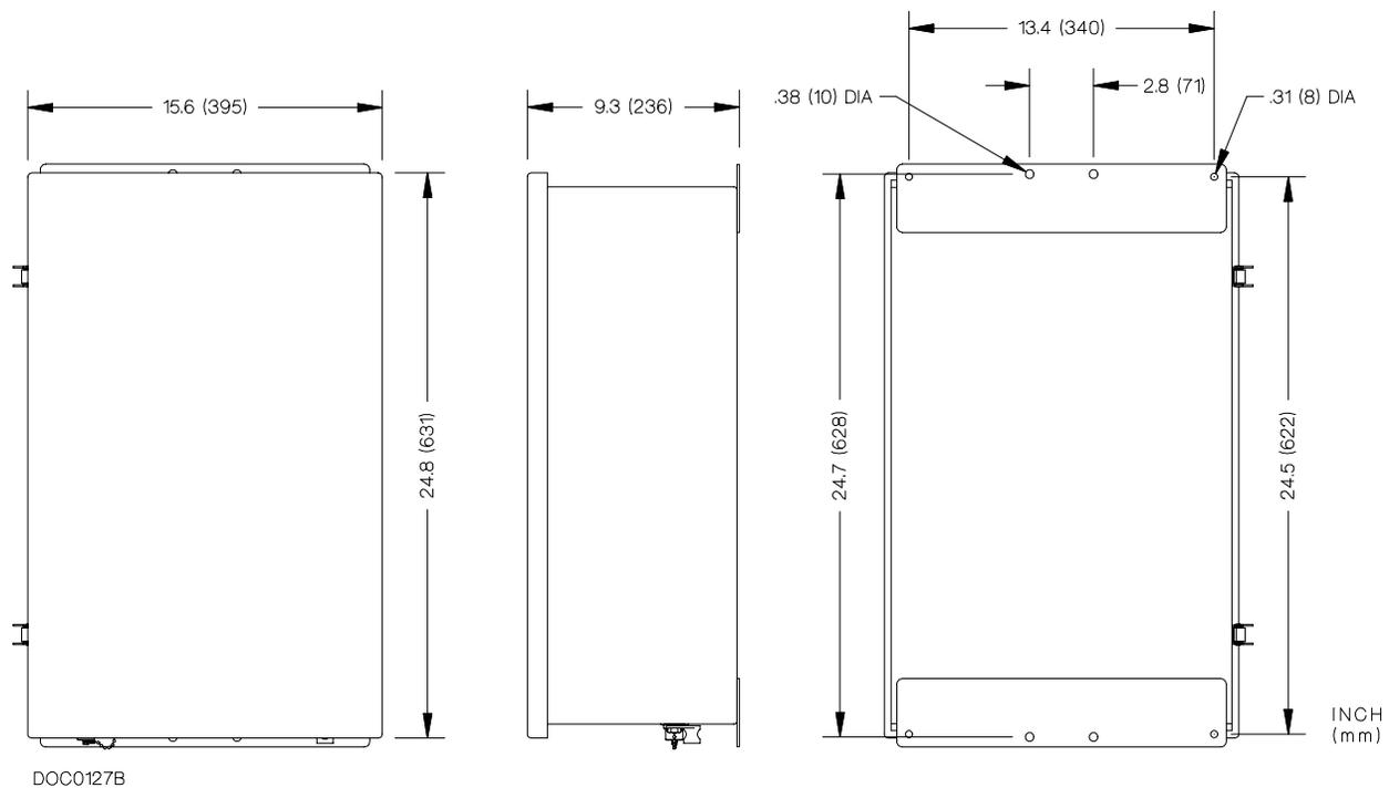
Figure 3-2. Small ROC Enclosure Dimensions
