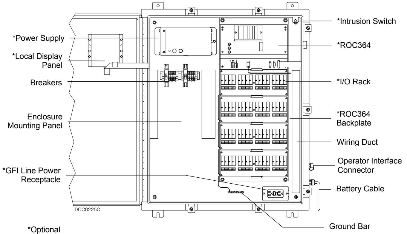
Figure 3-7. Large ROC Enclosure EN32 without Battery Compartment
