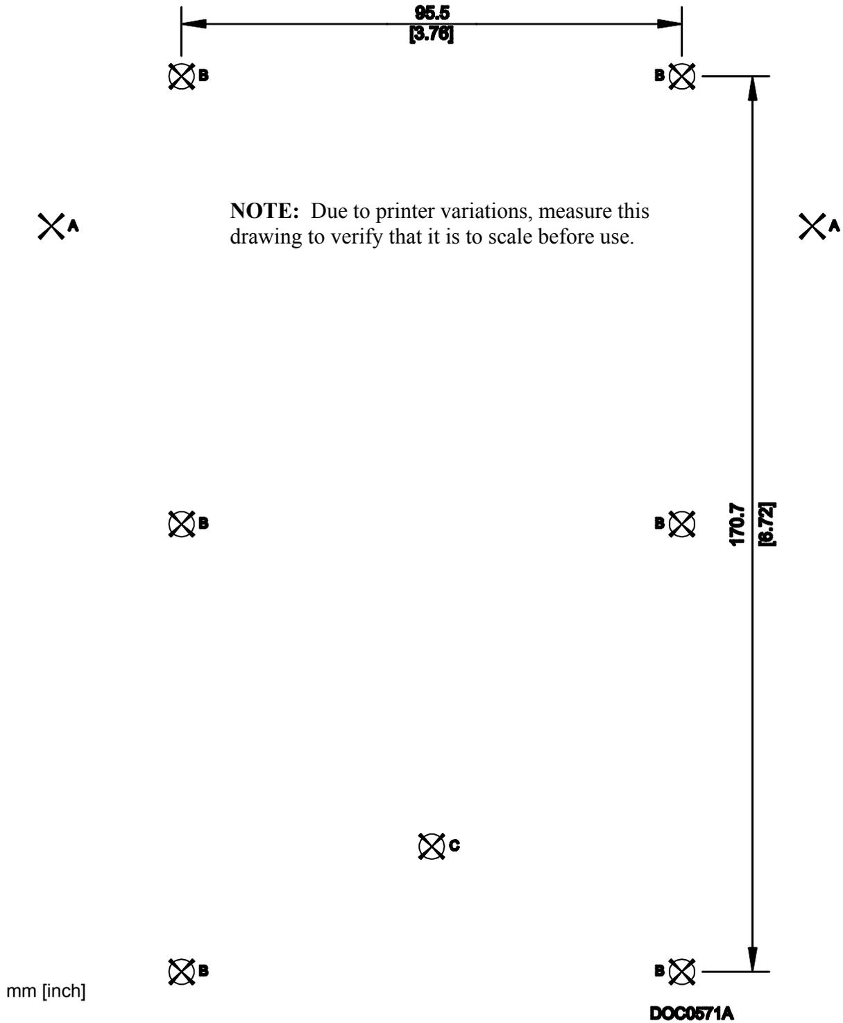
Figure 4-6. Enclosure Mounting Locations
