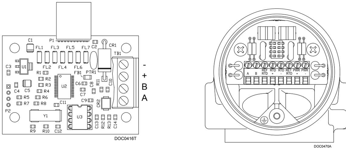
Figure 6-6. Terminations for a FloBoss 503 Remote MVS Installation
