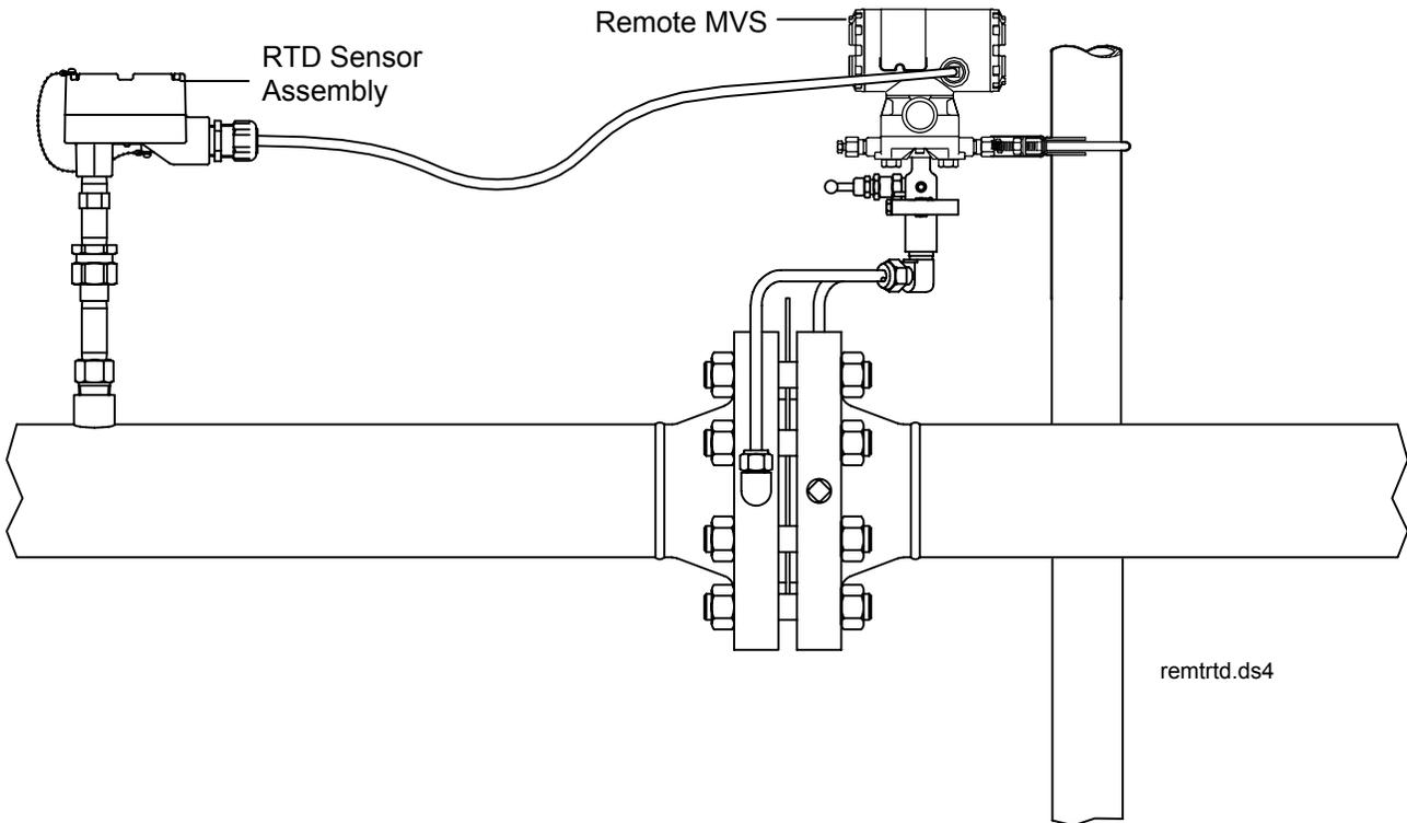
Figure 6-2. RTD Sensor Installed with Remote MVS (Class I Division 2 Installation Shown)
