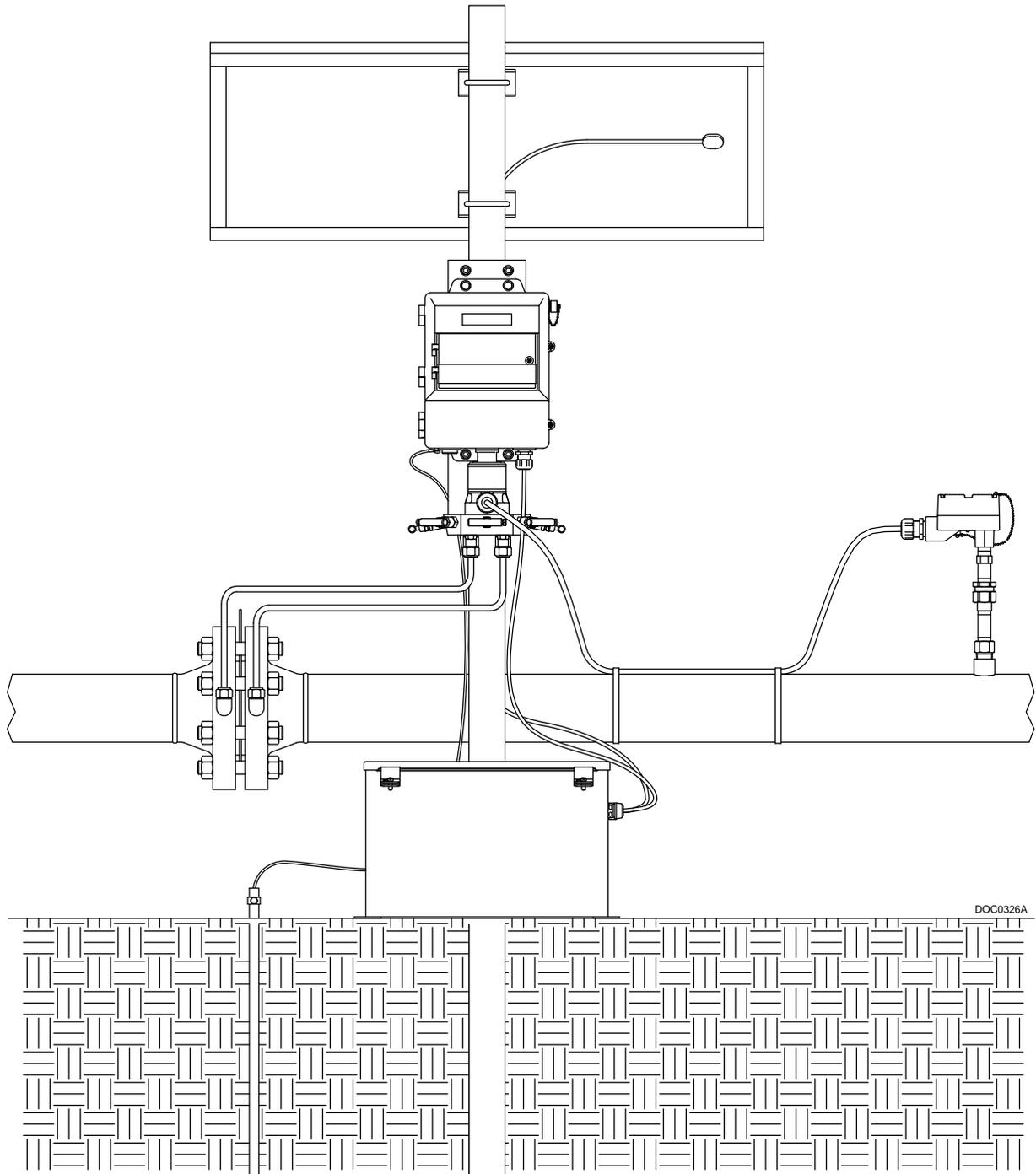
*Figure 5-2. Installation with Floor Mounted Battery Enclosure (FloBoss 407 Shown)*
