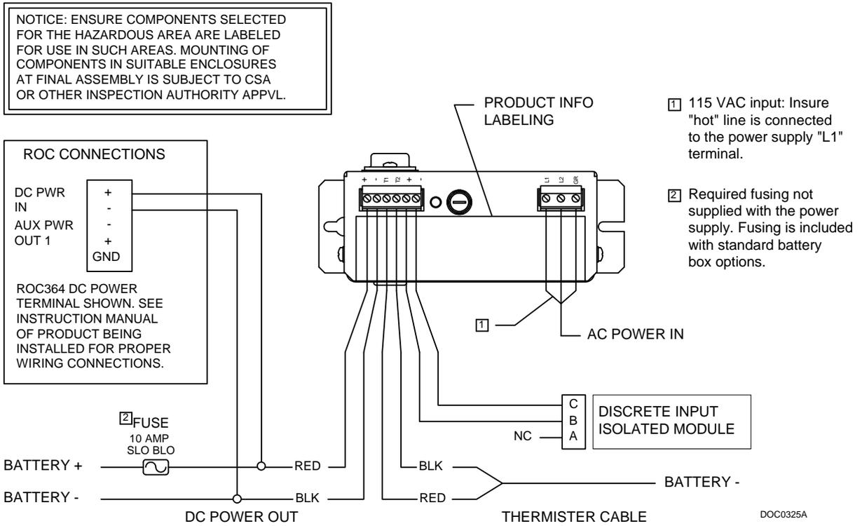
Figure 5-7. Low Current Power Supply Wiring
