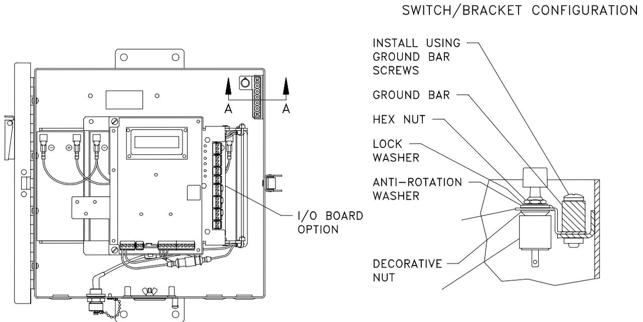
Figure 4-16. Intrusion Switch Mounting for FloBoss 500-Series Enclosures
