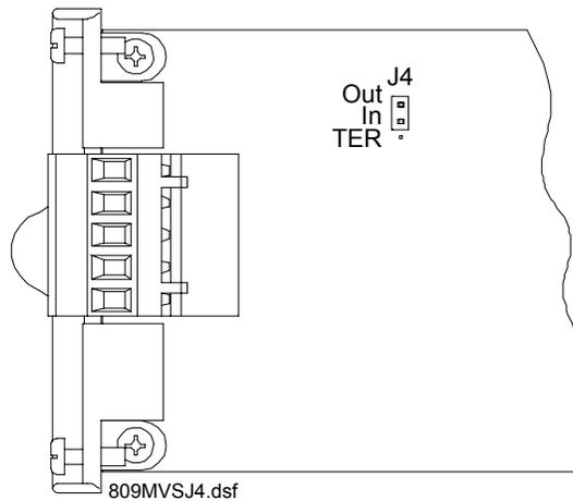
Figure 6-7. MVS Jumper J4 (Shown Not Terminated)
