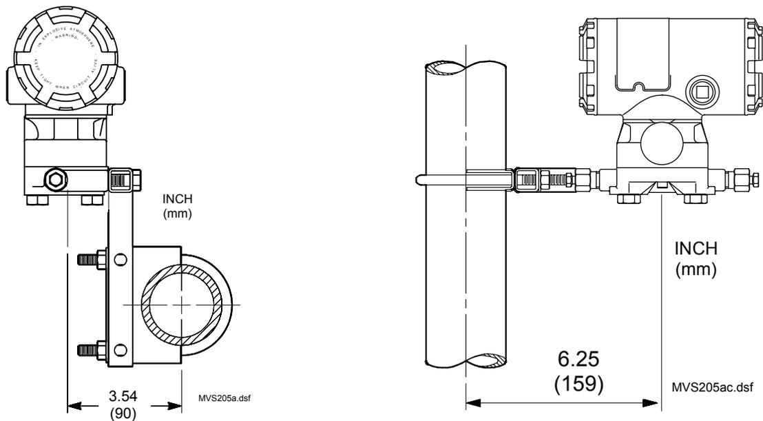
Figure 6-3. MVS205 Pipe Mounting (Horizontal and Vertical Pipe)
