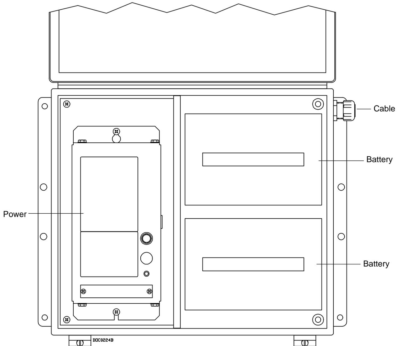
Figure 5-1. Battery Enclosure with Power Supply Compartment (Inside View)
