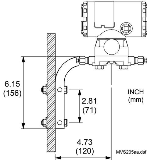
Figure 6-4. MVS205 Panel Mounting
