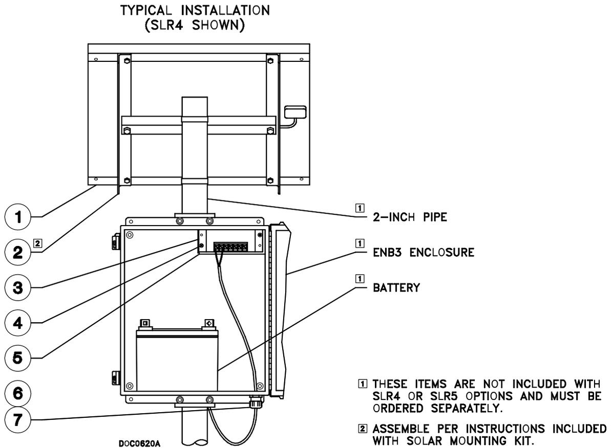
Figure 5-15. 20 Watt Solar Panel Mounting
