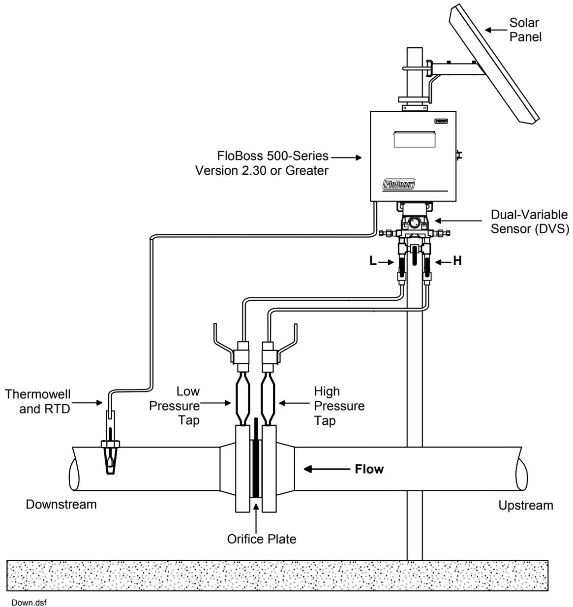
Figure 6-12. FloBoss 500-Series Version 2.30 or Greater – Downstream Process Connections
