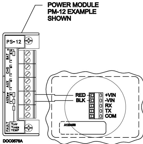
Figure 4-10. 12 Volts dc Power Input Module Wiring
