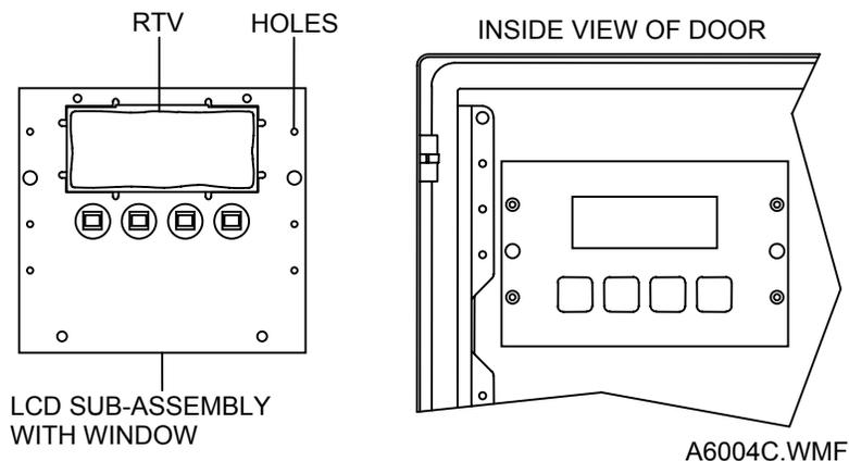
Figure 4-5. Using RTV to Seal Window
