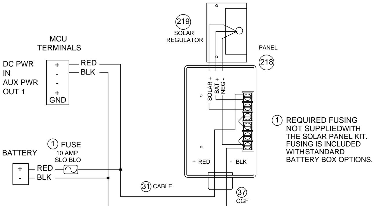
\* INSERT REGULATOR IN SOLAR PANEL JUNCTION BOX BEFORE CONNECTING TERMINALS
