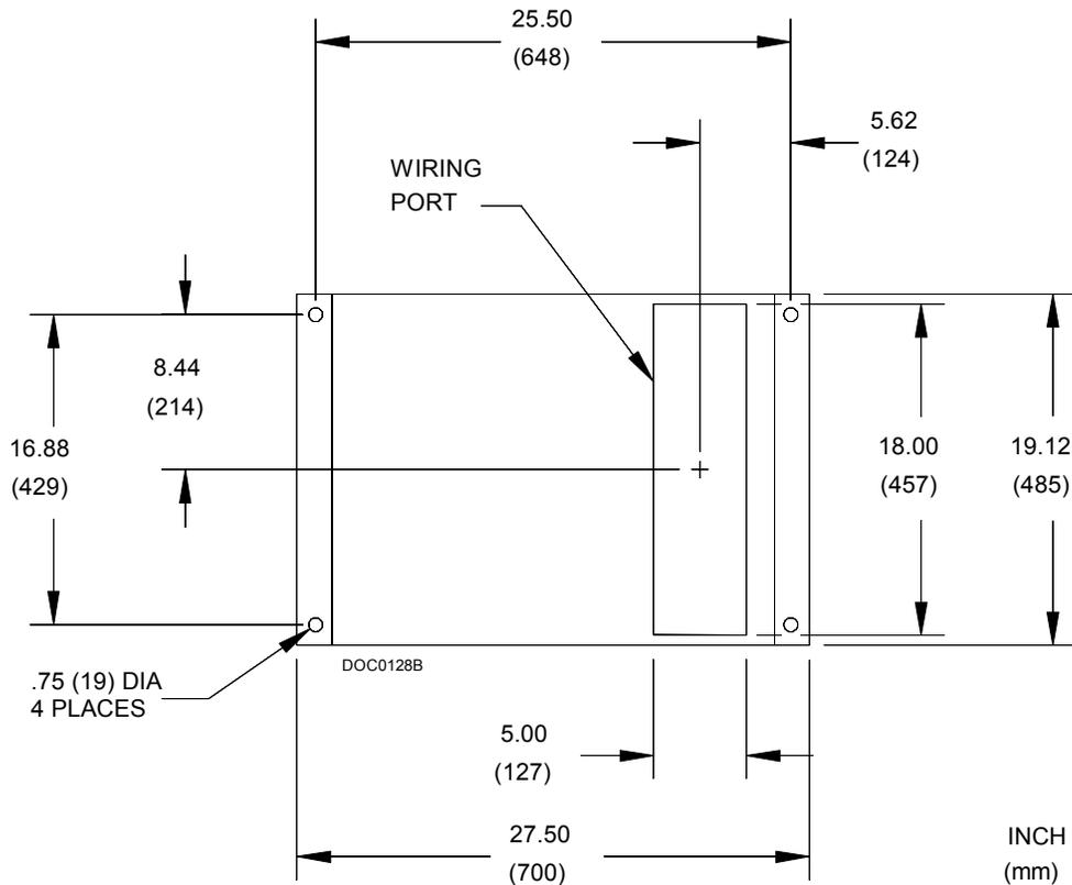
Figure 2-3. Base Bolt Pattern and Dimensions
