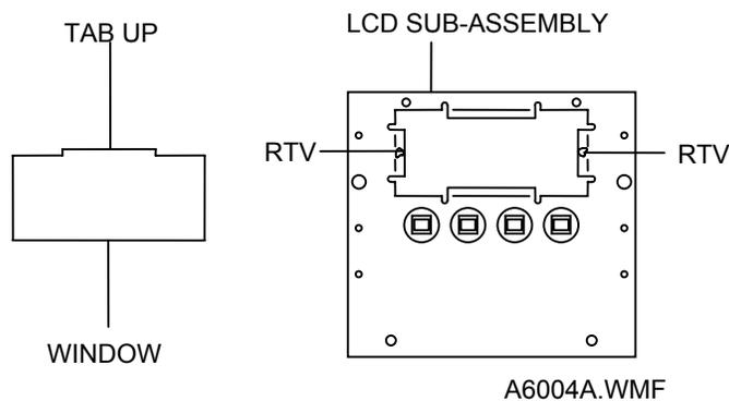
Figure 4-3. LCD Sub-Assembly
