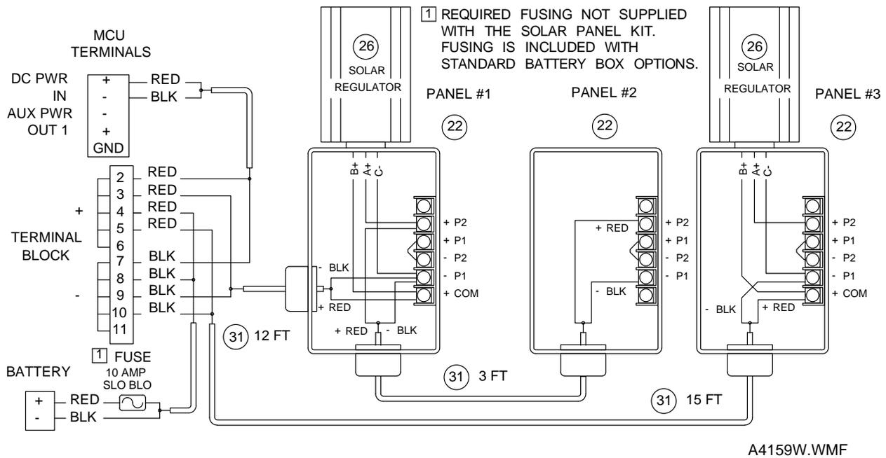
Figure 5-14. 60, 120, and 180-Watt Solar Panel Wiring
