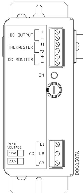
*Figure 5-5. Low Current Power Supply*
