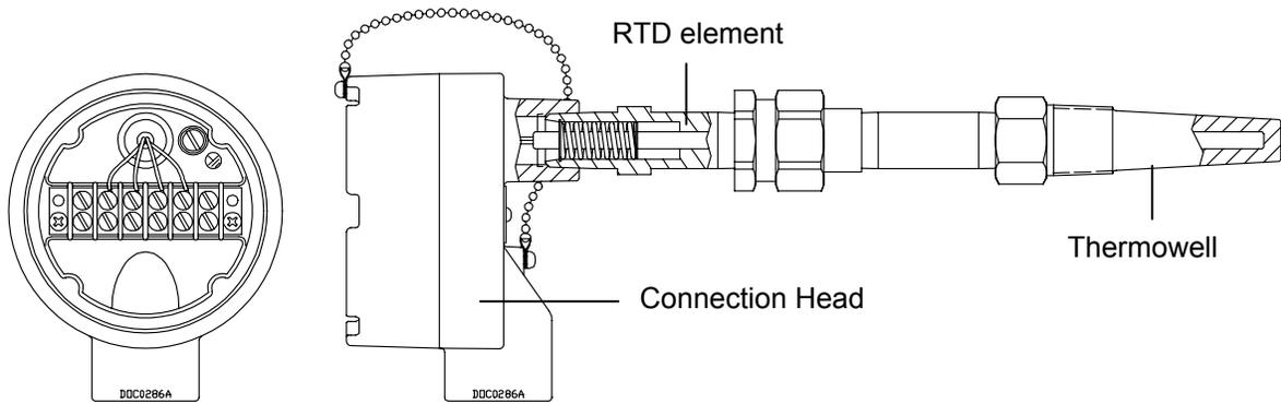
Figure 6-1. RTD Assembly Details
