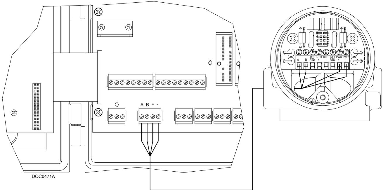
Figure 6-5. Signal Hook-Up for a FloBoss 407 Remote MVS Installation
