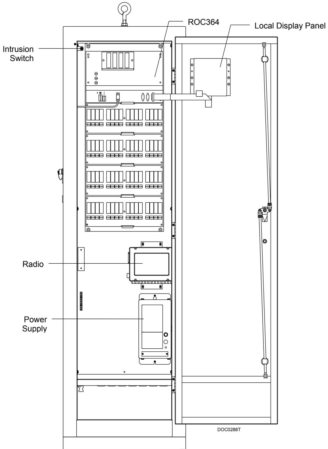
Figure 2-2. Typical Component Layout (ROC364 Shown)
