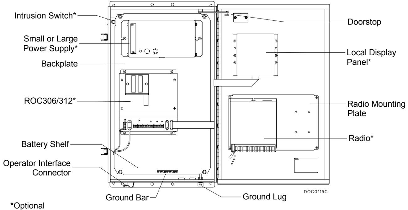
Figure 3-5. Model EN37 Mountable ROC Enclosure (Typical Component Layout)
