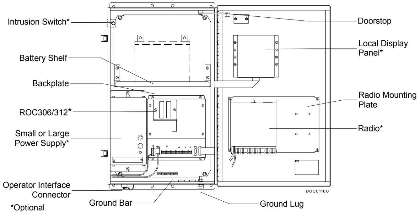
Figure 3-4. Model EN35 Mountable ROC Enclosure (Typical Component Layout)
