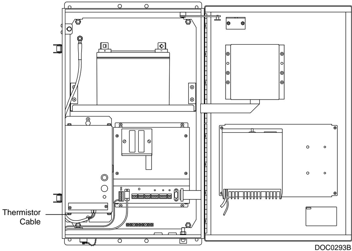
Figure 5-9. Thermistor Cable Location in Small ROC Enclosure
