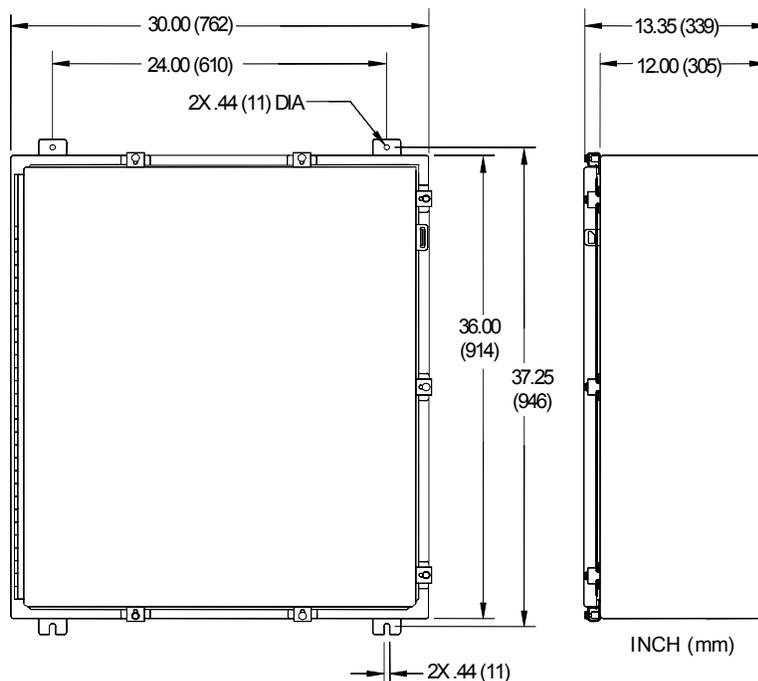
Figure 3-6. Large ROC Enclosure EN31 and EN32 Dimensions
