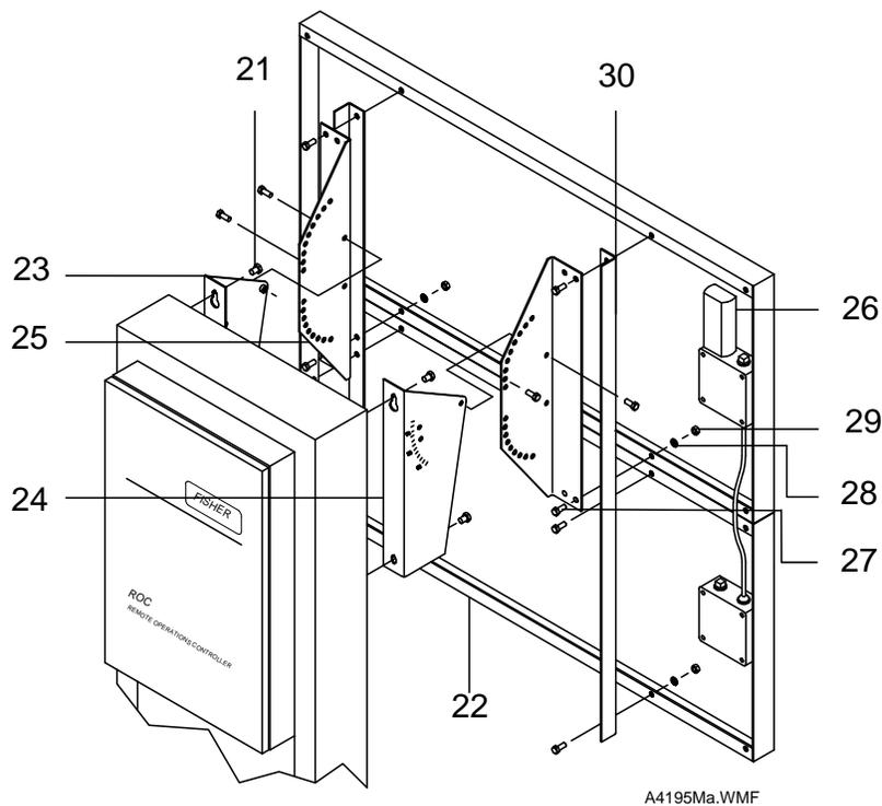
Figure 5-13. Solar Panel Mounting (120-Watt Shown)
