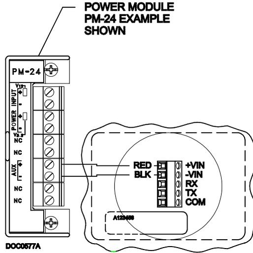
Figure 4-11. 24 Volts dc Power Input Module Wiring
