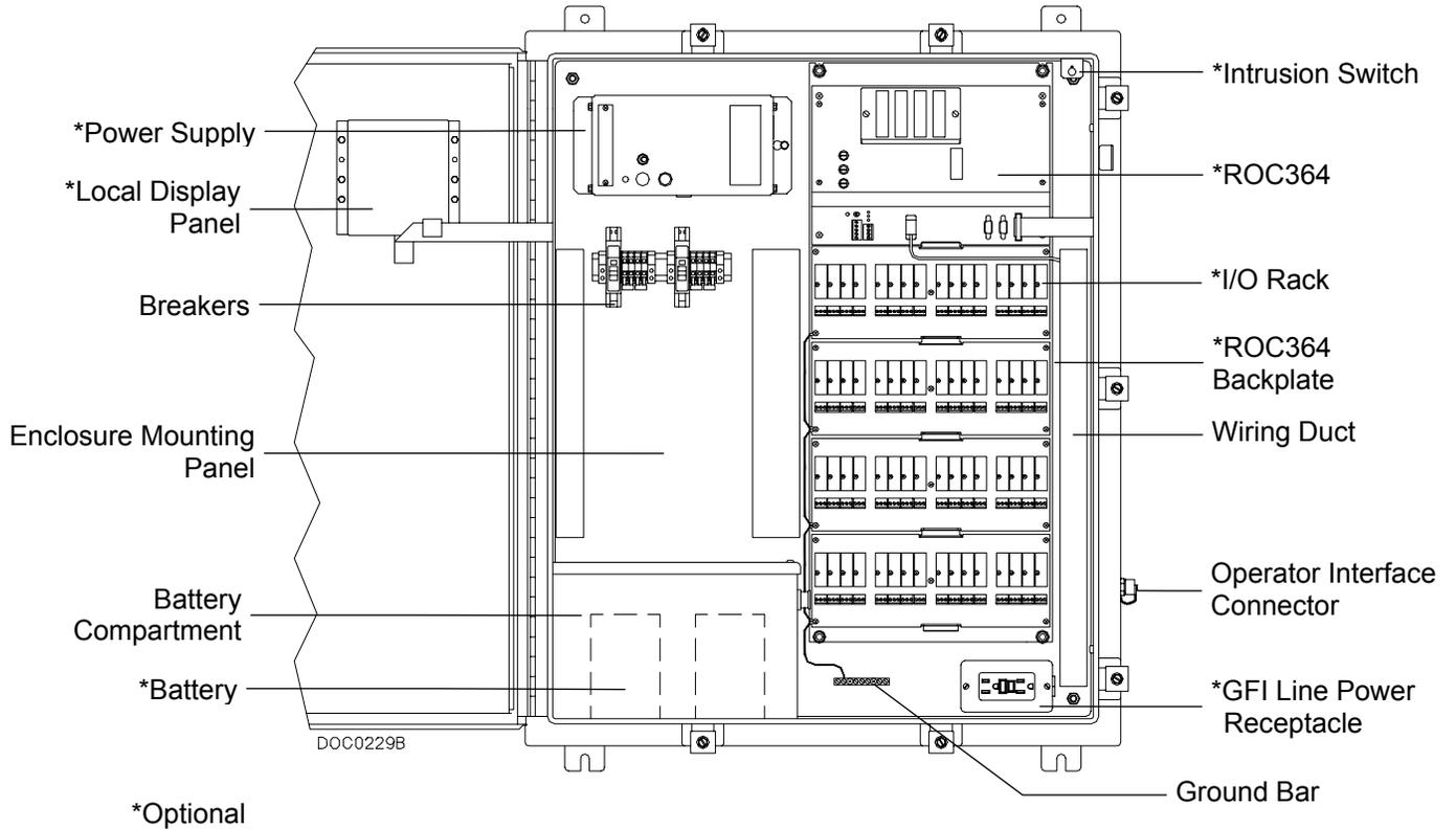
Figure 3-8. Large ROC Enclosure EN31 with Battery Compartment
