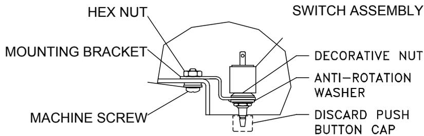
Figure 4-14. Intrusion Switch Mounting for EN23 Enclosures
