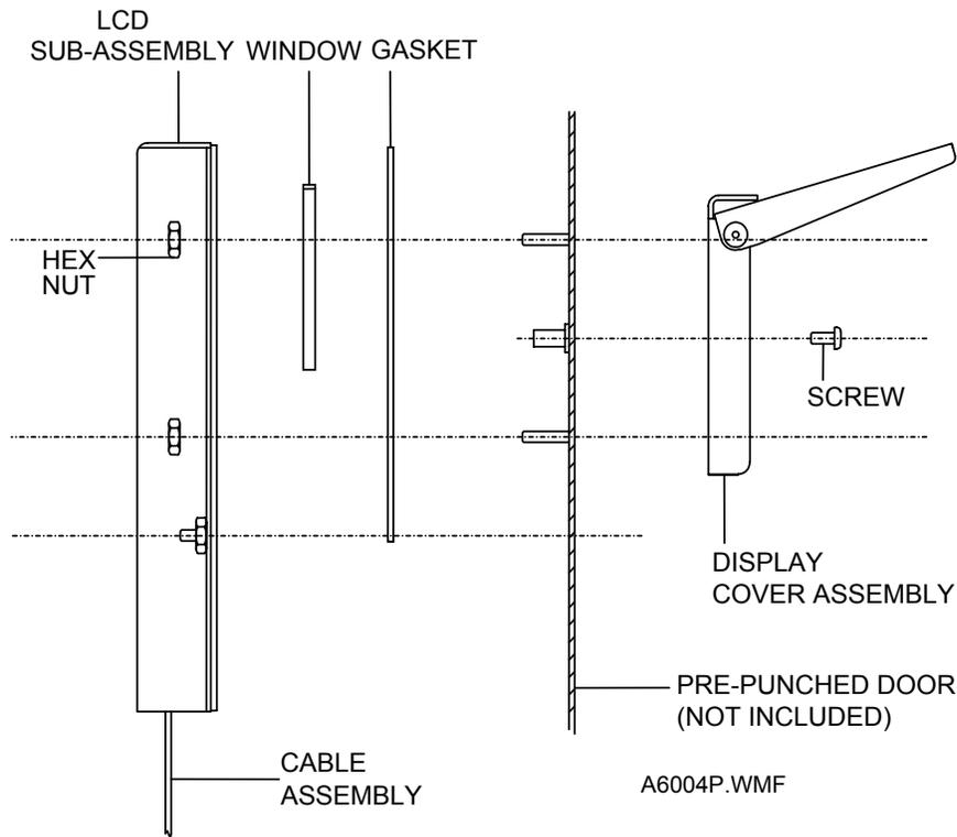
Figure 4-2. LDP Parts Orientation
