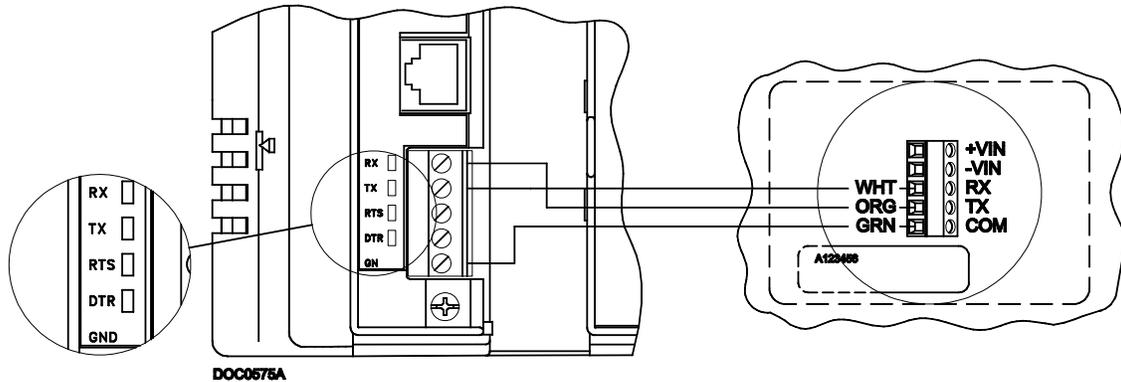
Figure 4-12. Communications Wiring (CPU Comm 2 Port Shown)
