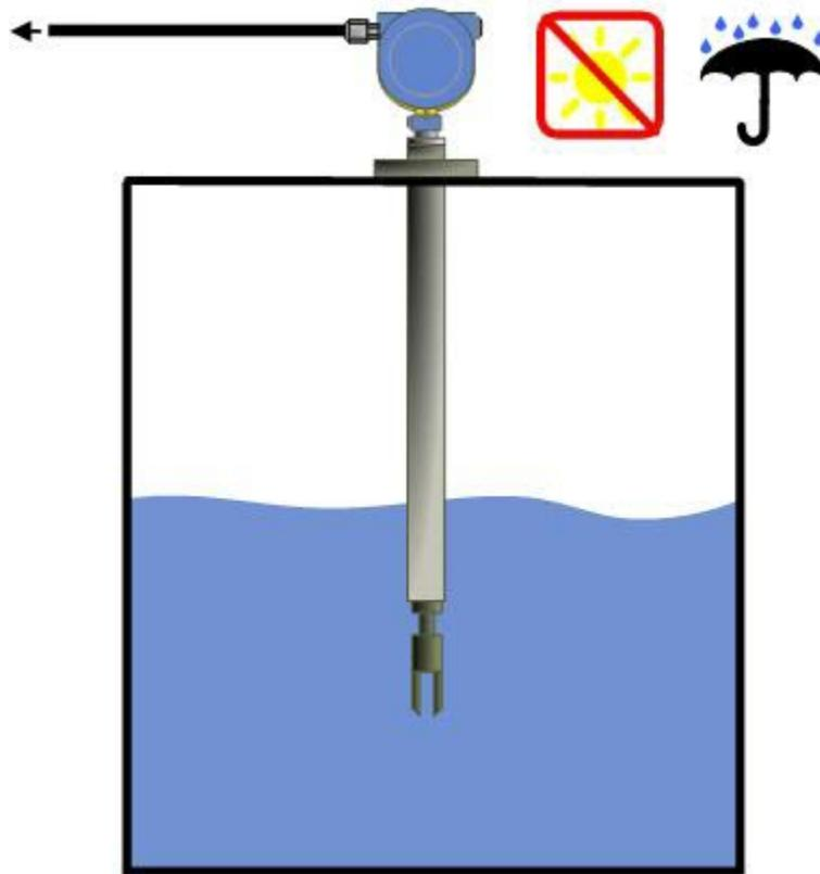
2. (Optional) To vary the insertion depth of the meter, mount the meter on a standoff section that attaches to the flange (not provided).
