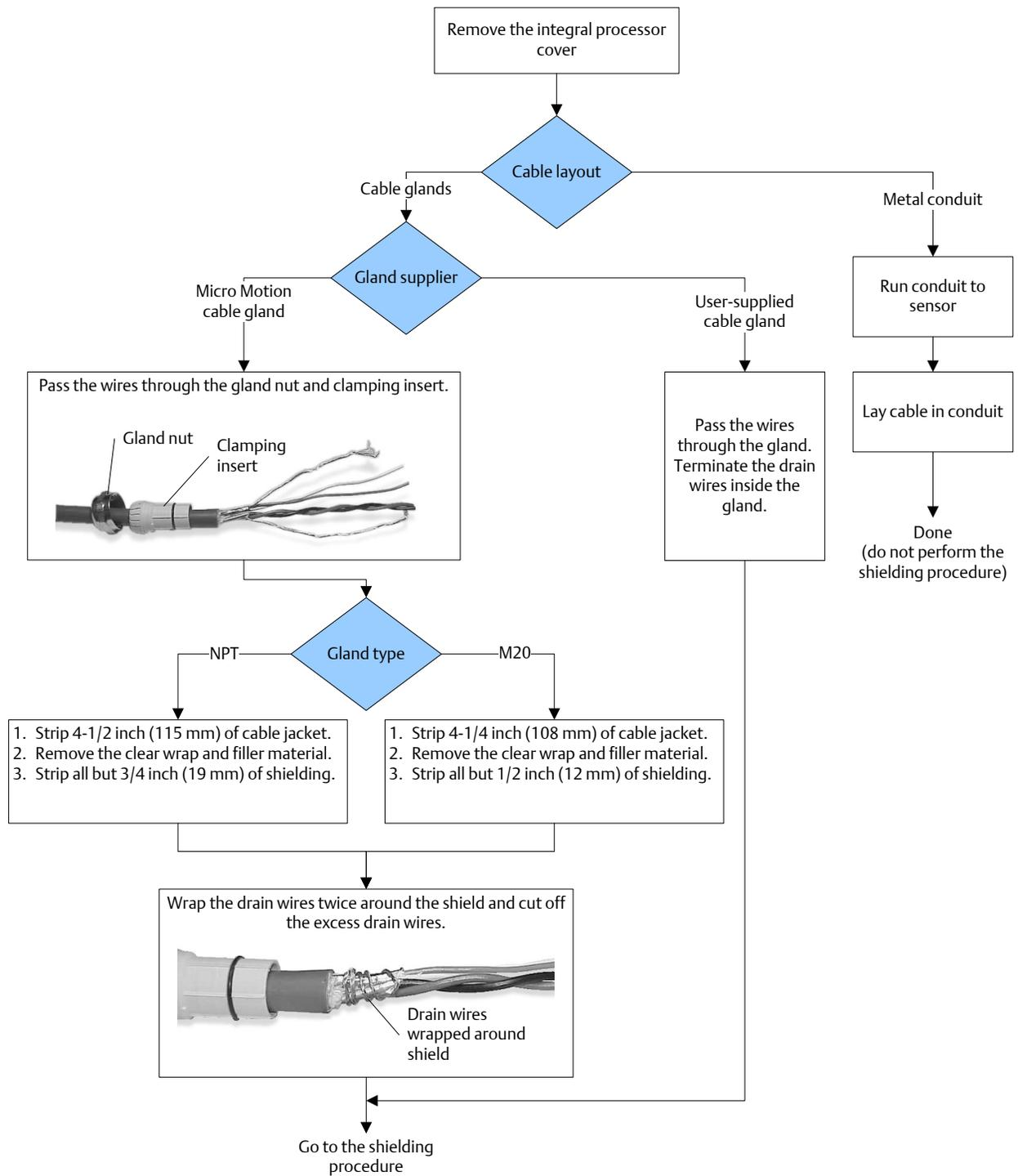
Figure 3-4: 4-wire cable shielding
