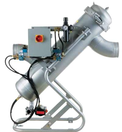
The MCS's magnetically coupled cleaning disc keeps the straining screen at optimal efficiency for continuous operation. This technology eliminates the need for dynamic seals, provides quick and easy access for maintenance, reduces potential leaks, and requires few moving parts while providing a long service life.
