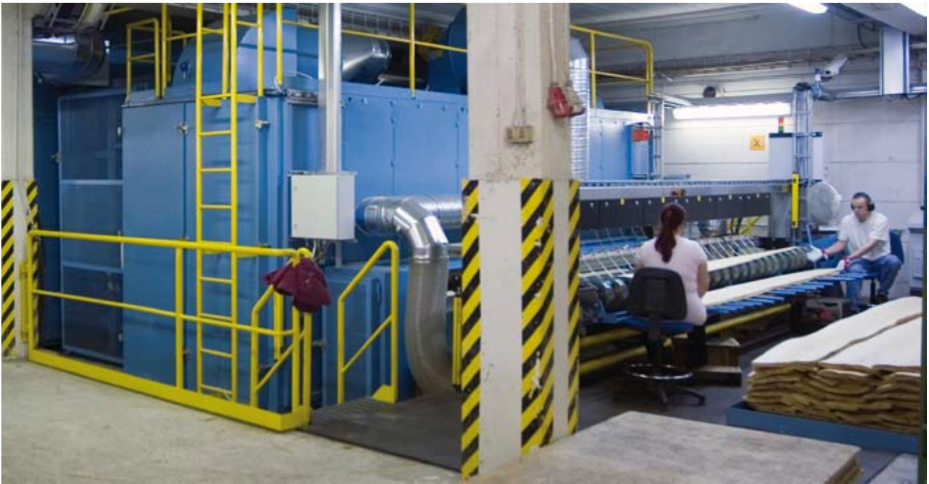
The veneer sheets are passed through the dryer and collected by operators at the end of the line.
