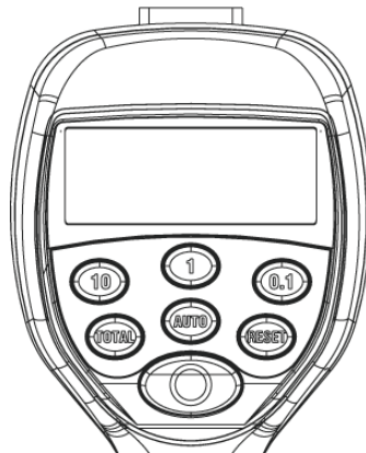
Figure 1: Meter button location
