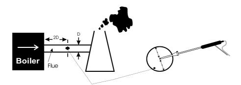
Use the probe's depth stop cone to fix it in flue diameters from  $^{1}/_{4}$  to  $^{4}/_{5}$  inch, 6 to 21 mm. Its maximum operating temperature is  $1112^{\circ}F / 600^{\circ}C$ .
