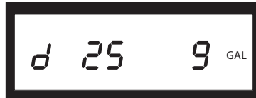
Figure 14: Meter type, digit resolution from the encoder and unit of measure
