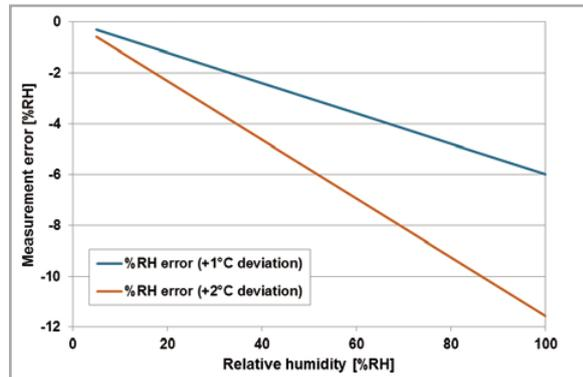
*Figure 1: Error in relative humidity reading resulting from +1°C (1.8°F) and +2°C (3.6°F) self-heating at room temperature (20°C, 68°F).*
