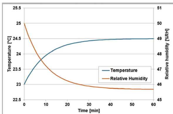
Figure 2: Example of a self-heating test. The transmitter is allowed to reach equilibrium with the surrounding environment.
