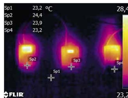
Figure 4: Transmitter temperatures 30 minutes after power-up.
