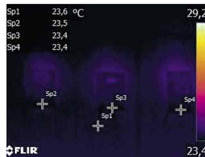
Figure 3: Transmitter temperatures before power-up.
