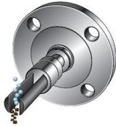
2. Size the T-piece so that the meter tines are retracted 1 in (25 mm) from the main pipe wall. For higher flow rates, increase this by 0.4 in (10 mm) for every 1 m/s increase in the main flow rate.
