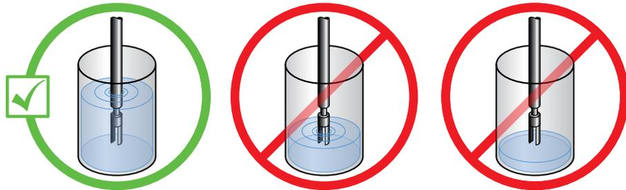
4. Confirm the meter tines are placed away from objects and disturbed flow.
