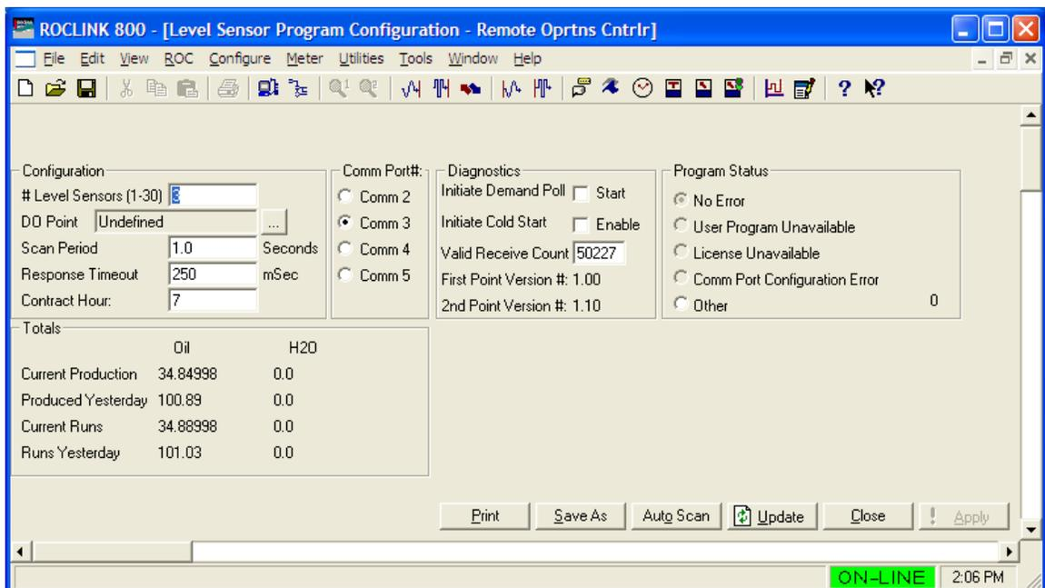
Figure 15. Level Sensor Program Configuration
