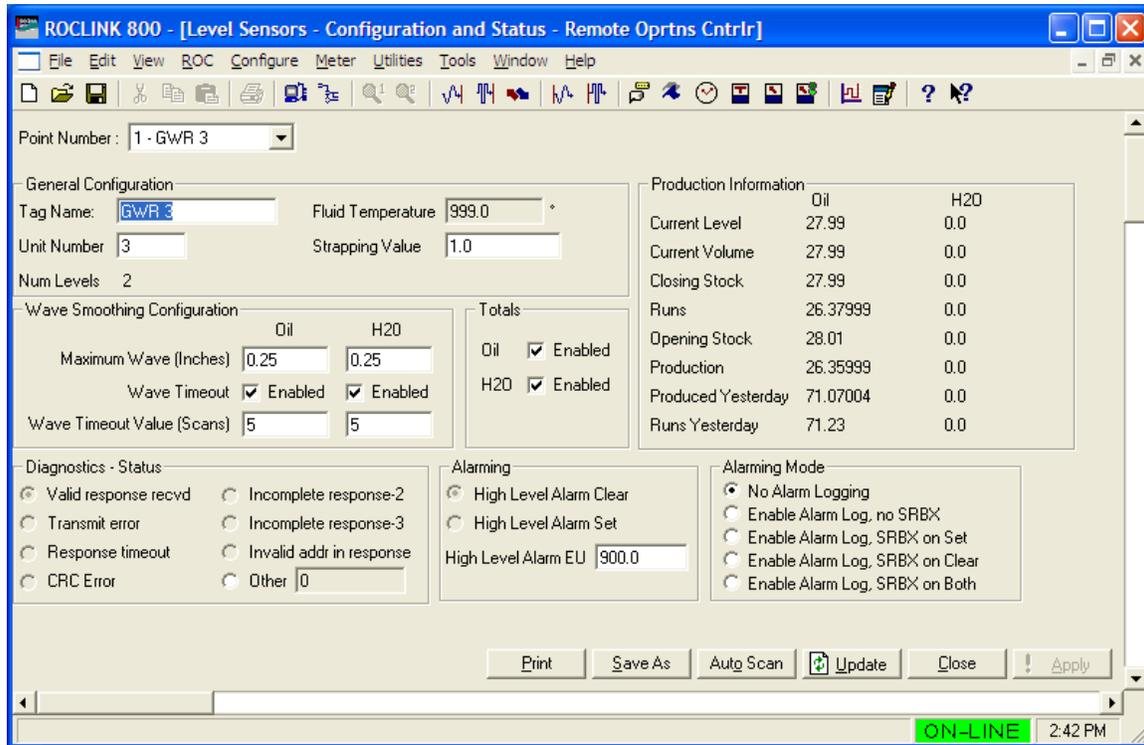
Figure 16. Level Sensors – Configuration and Status
