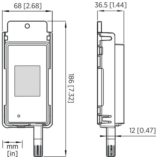
Figure 12 RFL100 Data Logger Dimensions with Mounting Bracket
