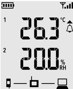
Figure 7 RFL100 with High Alarm Active on Channel 1
