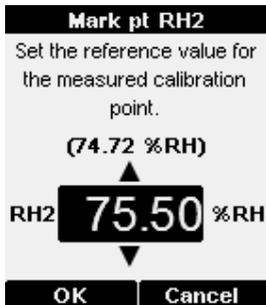
Correction to measurement at point 2 is now shown in the text for the menu item **[4] Point 2**.
