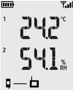
**Connected to an access point but viewLinc Enterprise Server not discovered yet:** Signal strength indicator
