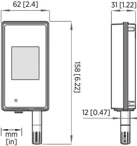
Figure 13 RFL100 Data Logger Dimensions
