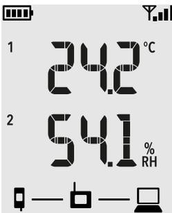
**Full connectivity:** Data logger has discovered a viewLinc Enterprise Server and is connected to it through the access point. You can now log in to the viewLinc Enterprise Server and accept the device to the system.
