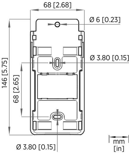
Figure 14 RFL100 Mounting Bracket Dimensions
