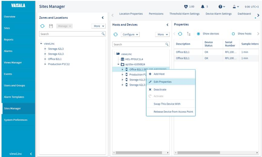
Figure 10 RFL100 Remote Management using viewLinc Enterprise Server
