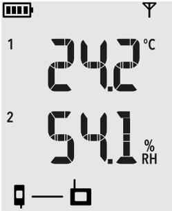
**Looking for an access point to join:** Line between data logger
