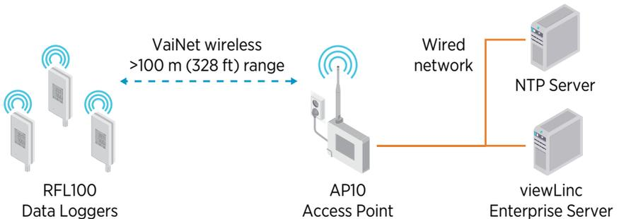
Figure 1 Connecting RFL100 to the viewLinc Monitoring System
