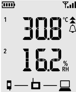
Figure 8 RFL100 with High-High Alarm Active on Channel 1
