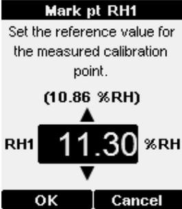
Correction to measurement at point 1 is now shown in the text for menu item **[3] Point 1**. If you are only doing a 1-point calibration, skip to [step 11](#).
