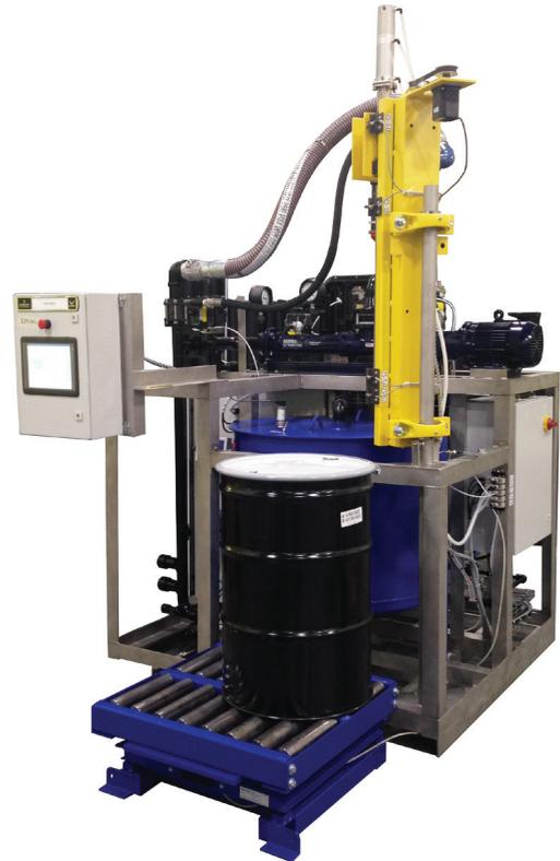
Emerson's newly enhanced Drum Decanting Unit is a compact solution with increased performance to decant the most viscous additives efficiently.
