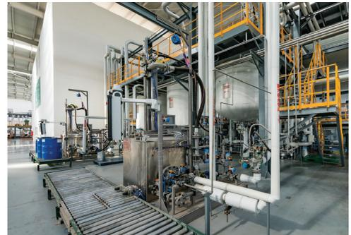
Emerson's Drum Decanting Units feature CIP technologies and can connect to piggyback lines to reduce cross-contamination between transfers. Photo courtesy of Copton.
