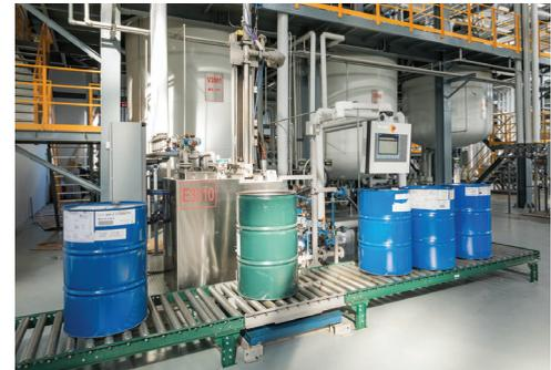
Emerson's Drum Decanting Units can automatically discharge components from drums and totes into a blender. Photo courtesy of Copton.
