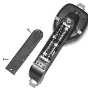
Figure 18: Replacing the batteries
