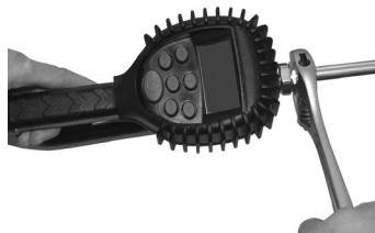
Figure 6: Tighten nozzle with wrench
