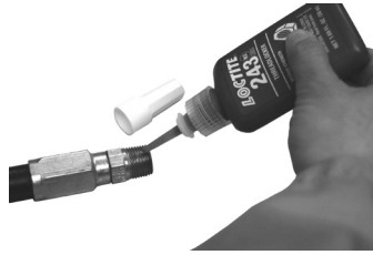
Figure 2: Apply thread sealant
