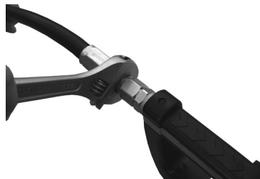
Figure 4: Use wrench to tighten
