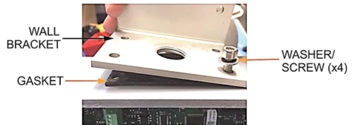
Figure 6: M5000 gasket on amplifier
