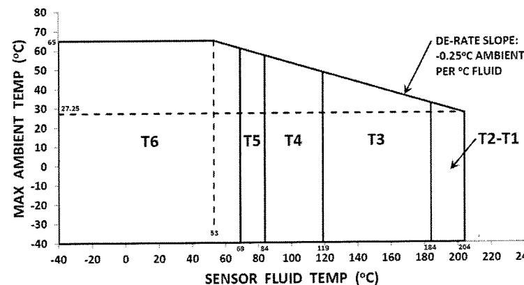
Note: Use the above graph to determine the temperature class for a given fluid and ambient temperature.
