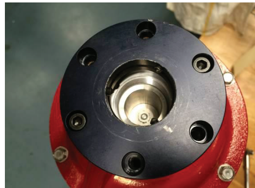
Figure 10: Set screws (shown advanced for clarification)
