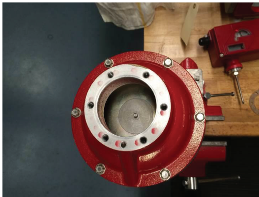
Figure 1: Actuator with locknut and washer removed
