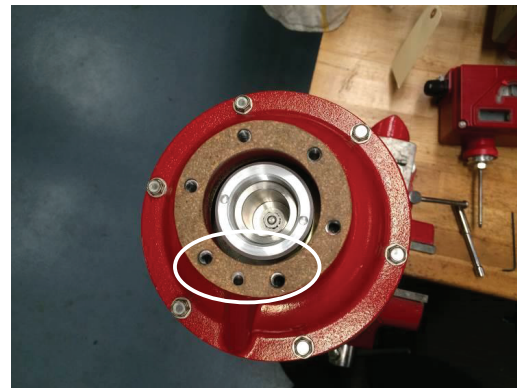
Figure 5: Gasket installation
