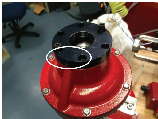
Figure 6: Adapter ring installation
