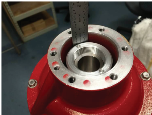
Figure 4: Actuator with shell and stop installed
