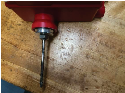
Figure 9: Positioner plunger and groove
