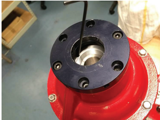
Figure 7: Setting the actuator travel
