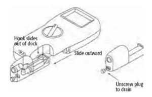
NOTE: CO2 reading will be low if the Water Trap Plug is not in place.
