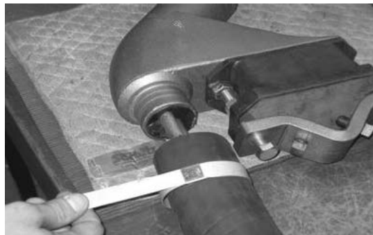
Figure 23: Install protective hose
