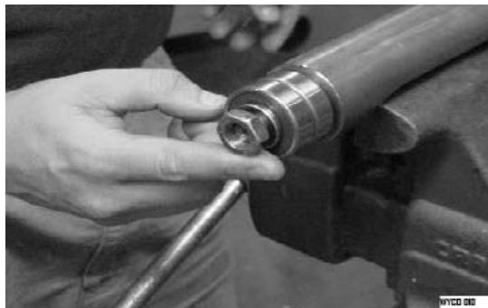
Figure 7: Tighten hex nut
