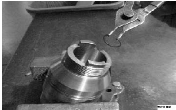
Figure 13: Remove retaining ring
