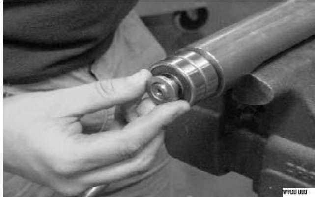
Figure 6: Slide washer onto rotor
