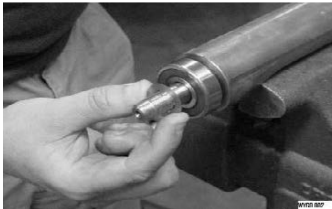
Figure 5: Slide shim onto rotor
