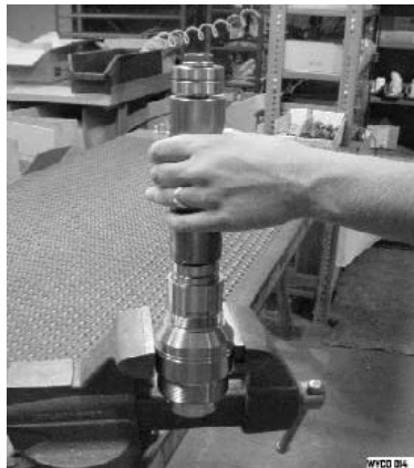
Figure 9: Clamp motor housing in vise
