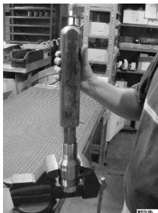
Figure 10: Slide head housing over rotor
