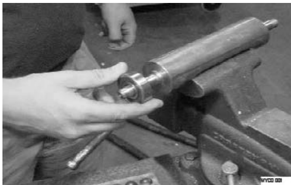
Figure 4: Slide bearing onto rotor
