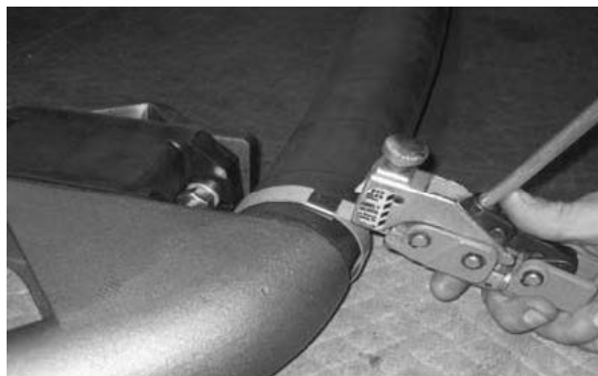
Figure 24: Punch lock clamp
