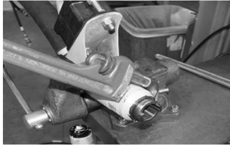
Figure 18: Unscrew motor housing
