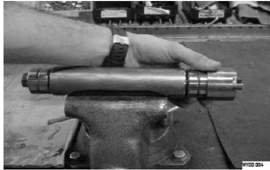
Figure 8: Install upper bearing cup
