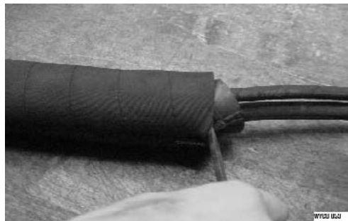
Figure 16: Remove rubber plug
