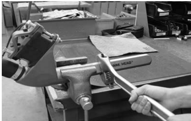
Figure 12: Tighten head housing
