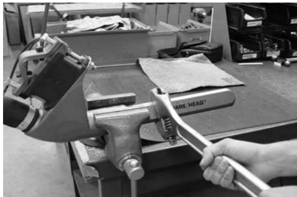
Figure 1: Loosen square head housing
