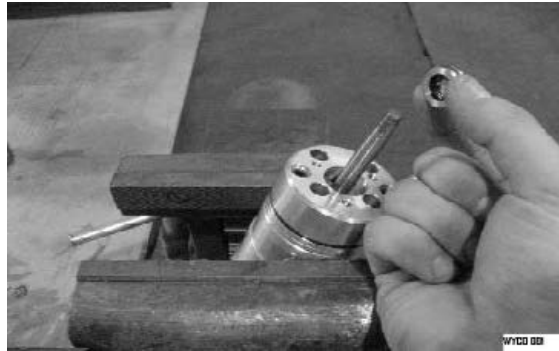
Figure 15: Press seal into motor
