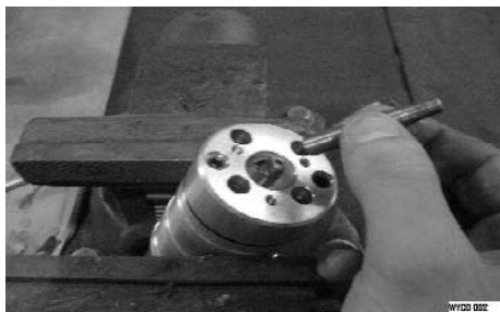
Figure 14: Place tapered guide
