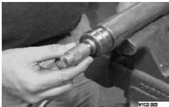
Figure 3: Unscrew driver sleeve
