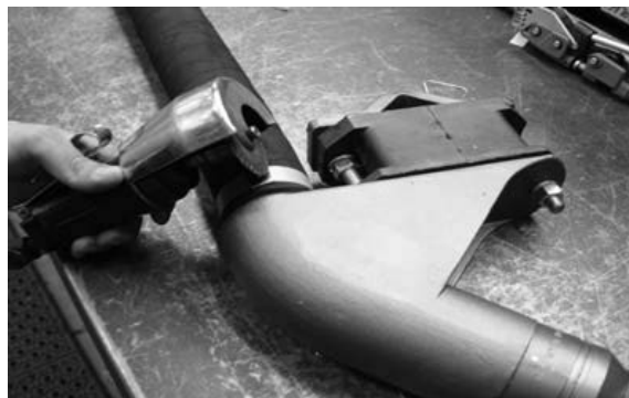
Figure 17: Loosen hose clamp
