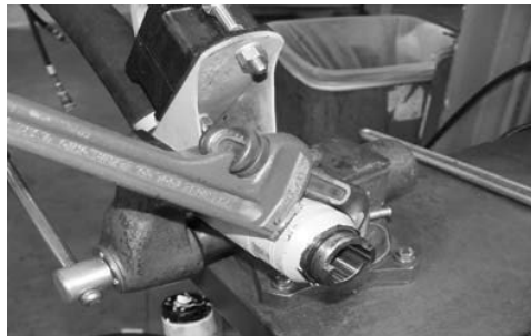
Figure 21: Tighten motor housing
