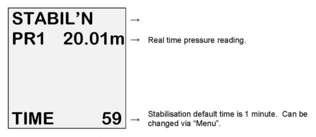
When complete press of to start the tightness test:
