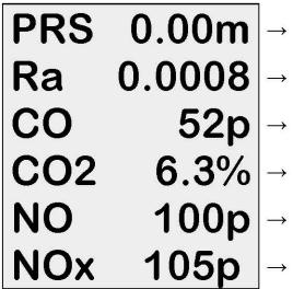
The AUX (auxillary) display can be customised via MENU / SCREEN / AUX.
