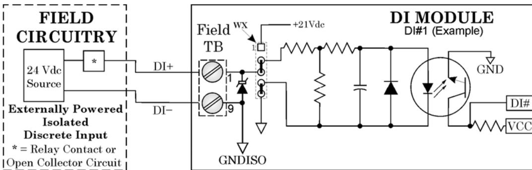
Figure 3-8. Externally Powered DI Module - Wiring Diagram
