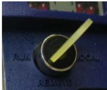
*Figure 4-2. Run/Remote/Local Key Switch*
