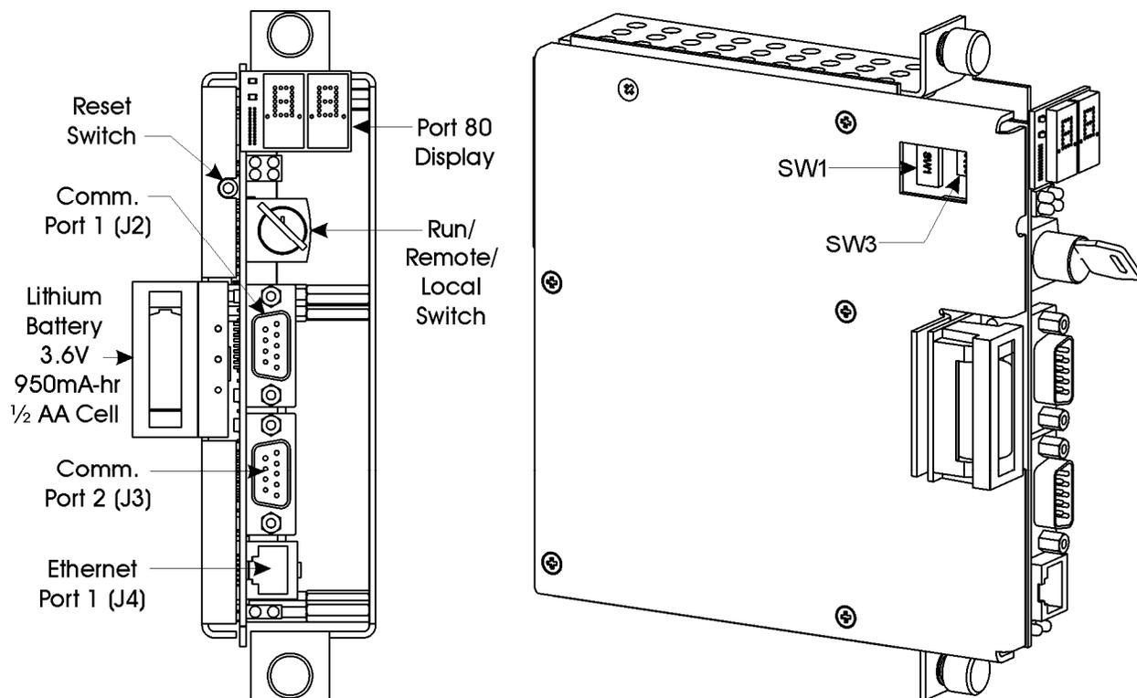
Figure 2-12. ControlWave CPU Module (without SCB)
