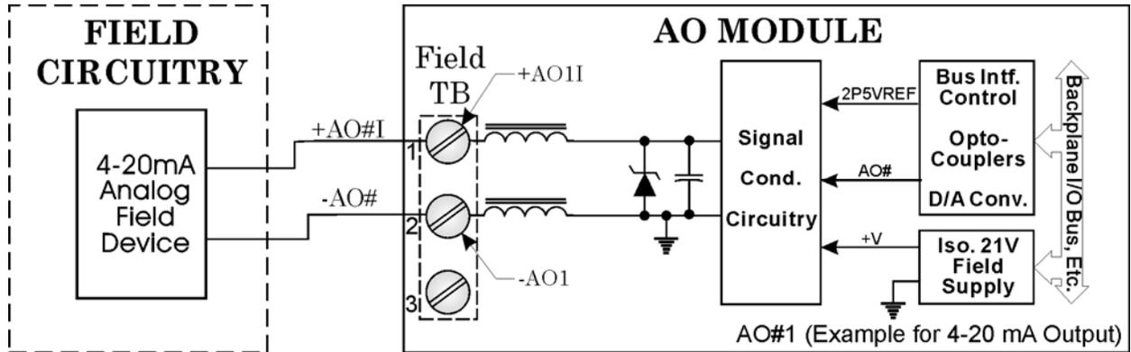
Figure 3-23. 4-20mA Current Loop AO - Wiring Diagrams
