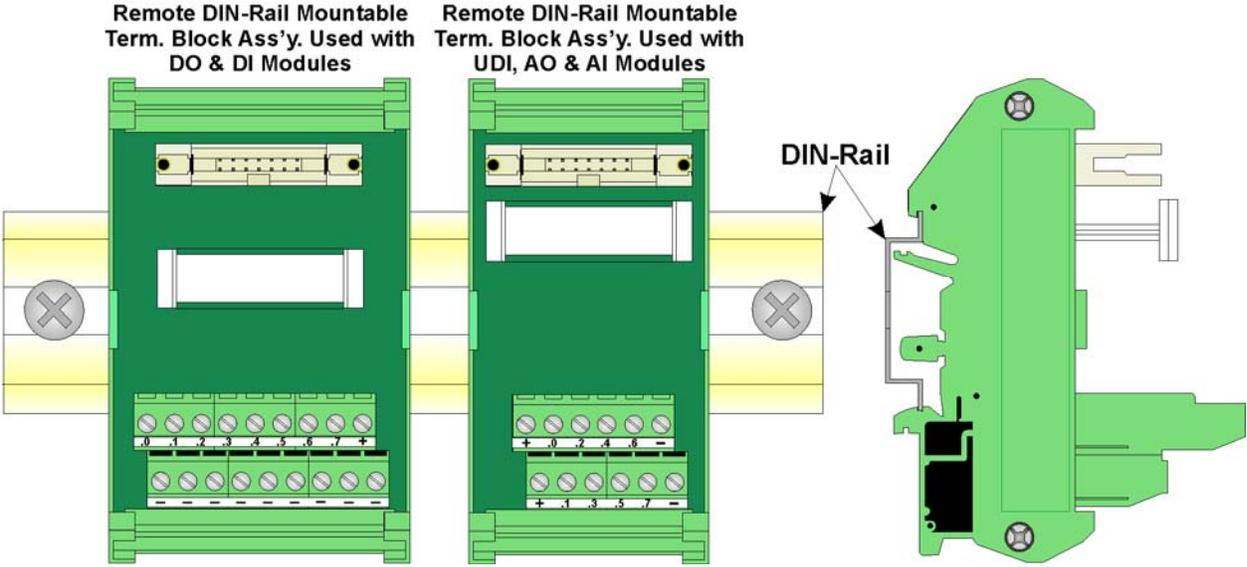
Figure 3-4. I/O Module (Remote Termination) Wire Routing
