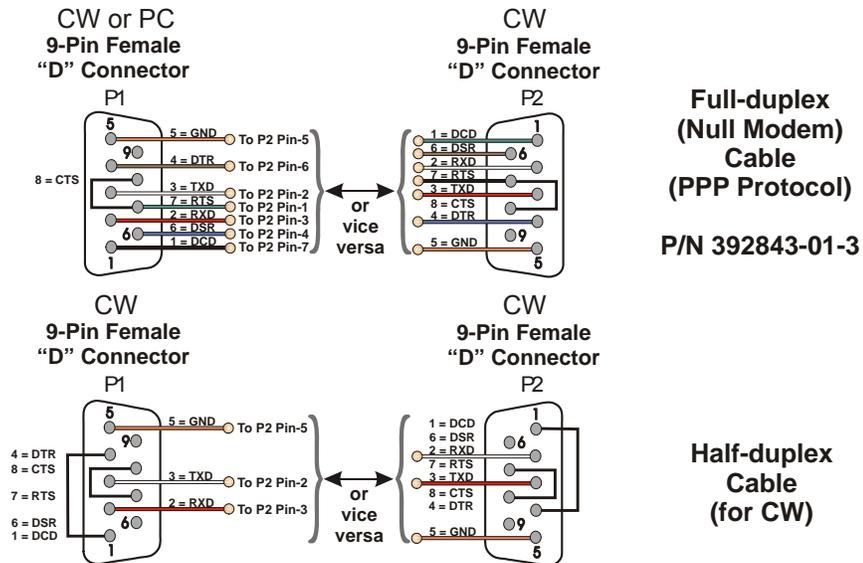
Figure 2-15. Full-duplex and Half-duplex Cable
