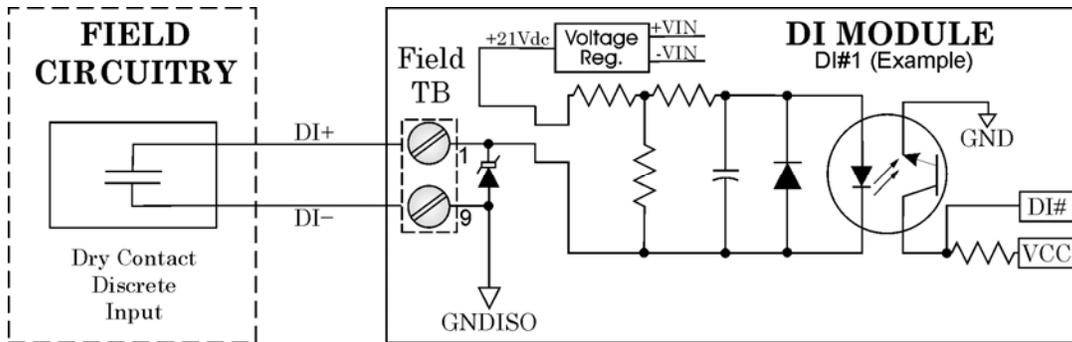
Figure 3-7. Internally Sourced DI Module - Wiring Diagram
