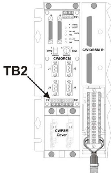
Figure 2-11. Location of TB2 on ControlWave I/O Switcher
