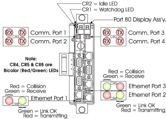
Figure 5-11. CPU Module (CPU & SCB boards) Port & LED Designations
