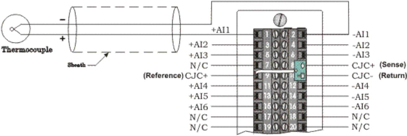
*Figure 3-33. Isolated Thermocouple Module - Wiring Diagram*
