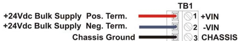
*Figure 2-6. Wiring System Power to the PSSM*
