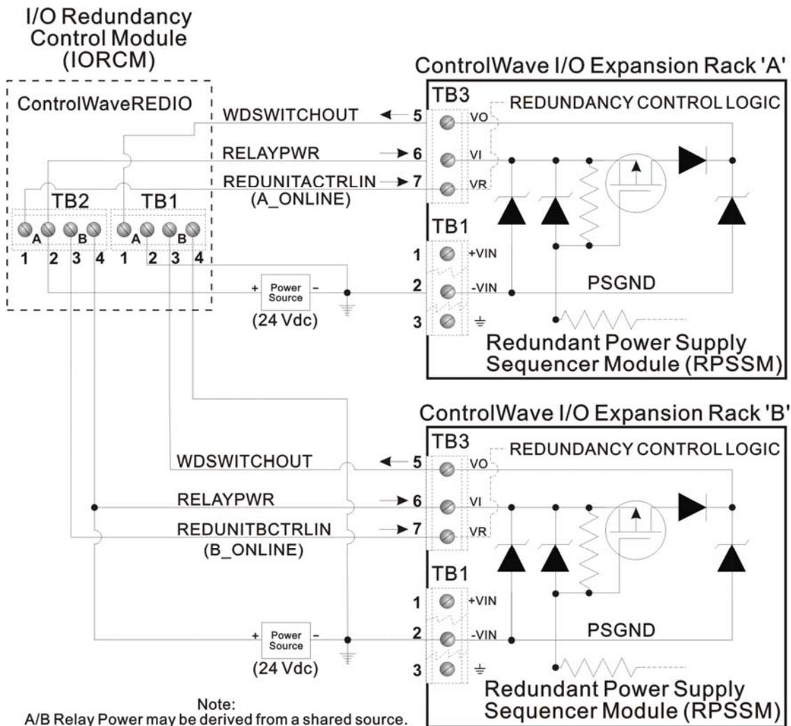
*Figure 2-10. ControlWave to ControlWave REDI/O - Redundancy Field Wiring*
