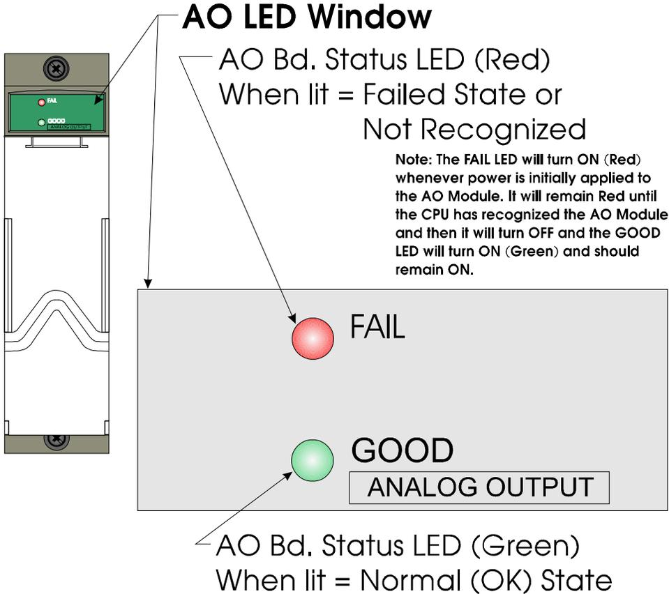
Figure 5-13. Analog Output (AO) Module LED Designations
