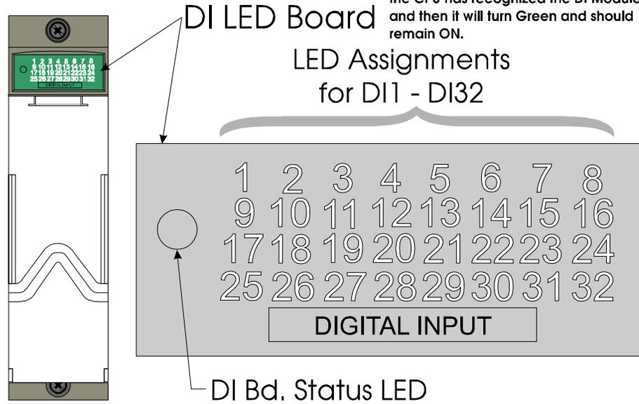
Figure 5-14. Digital Input (DI) Module LED Designations
