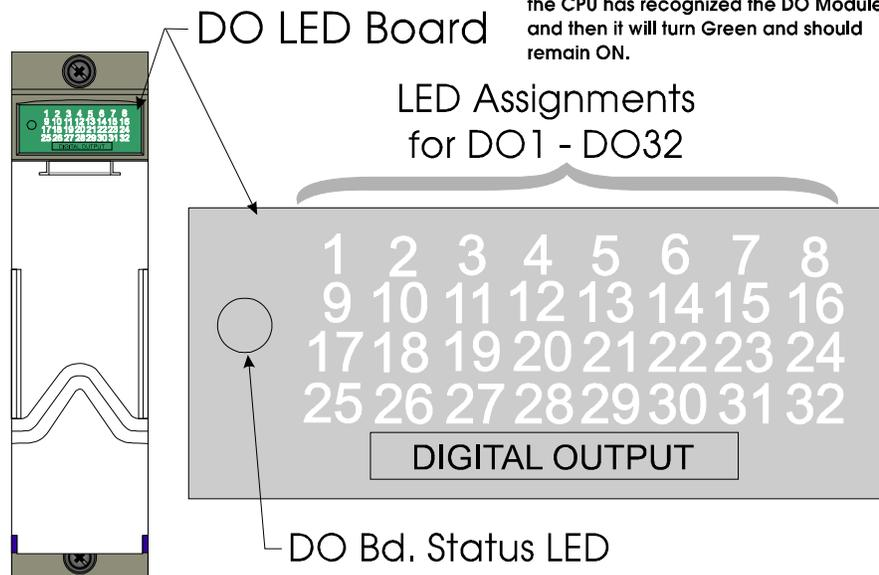
Figure 5-15. Digital Output (DO) Module LED Designations
