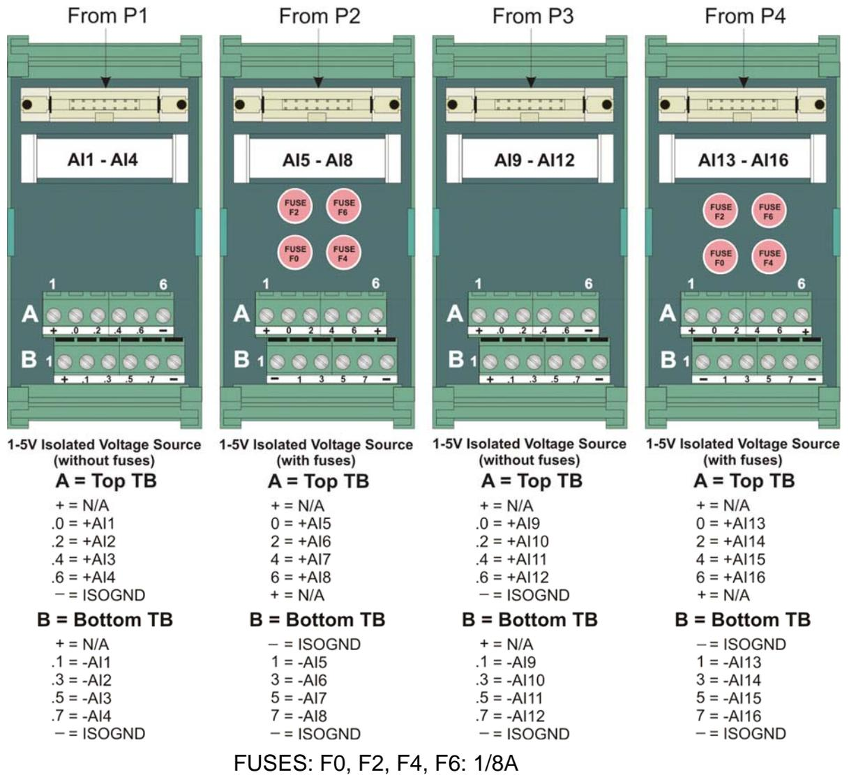
Figure 3-20. Remote DIN-Rail Mountable Terminal Block Assembly Assignments for 1-5V AI Operation
