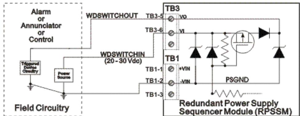
Figure 2-9. Watchdog Switch Field Wiring
