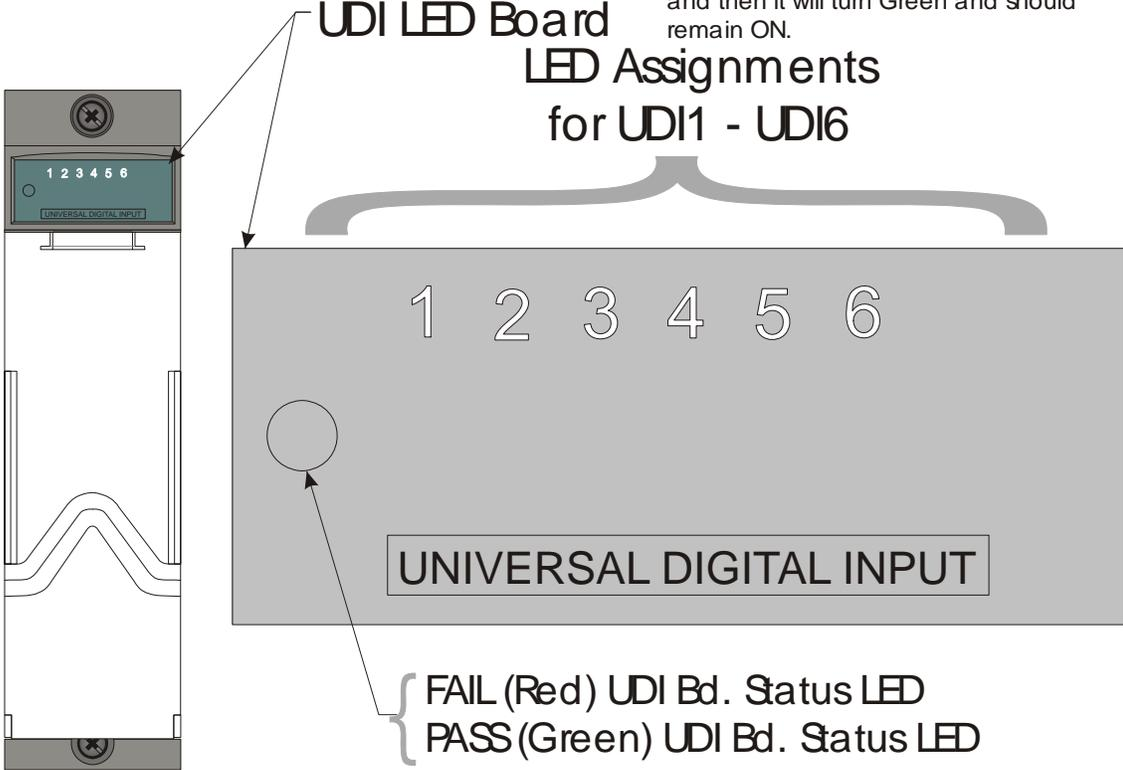
Figure 5-16. Universal Digital Input (UDI) Module LED Designations
