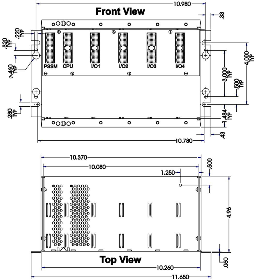
Figure 2-2. 4-I/O Module ControlWave - Mounting Diagram
