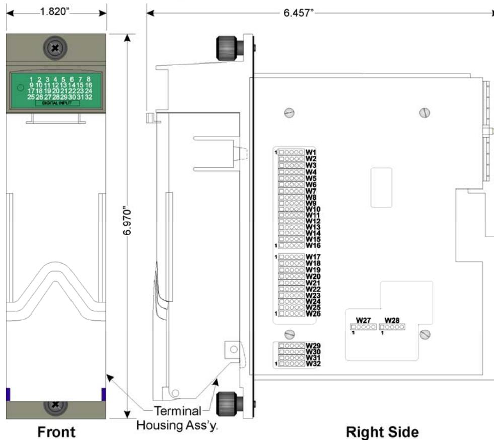
Figure 3-5. DI Module -Right Side View - Jumper Locations
