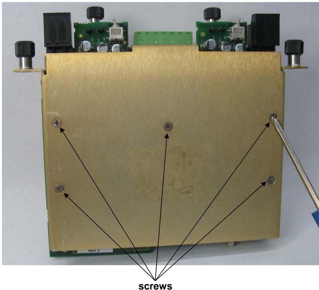
*Figure 2-4. Removing the Protective Case from the PSSM*
