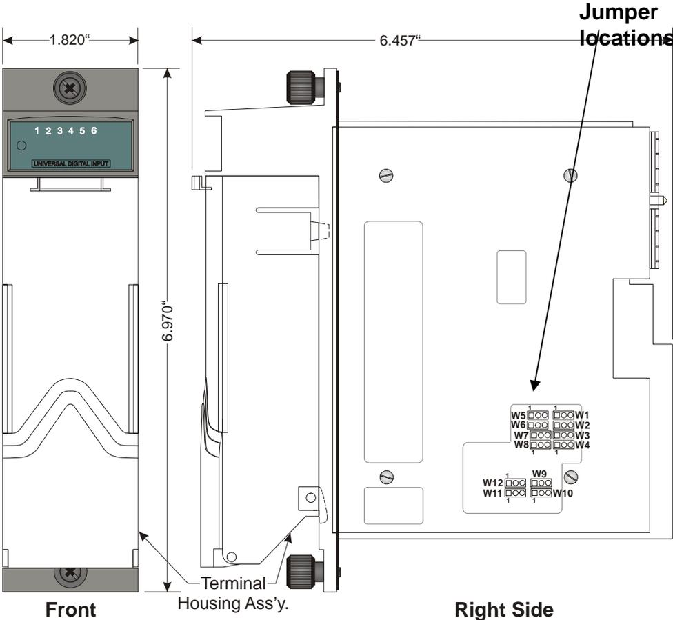
*Figure 3-24. - UDI Module -Right Side View -Jumper Locations*
