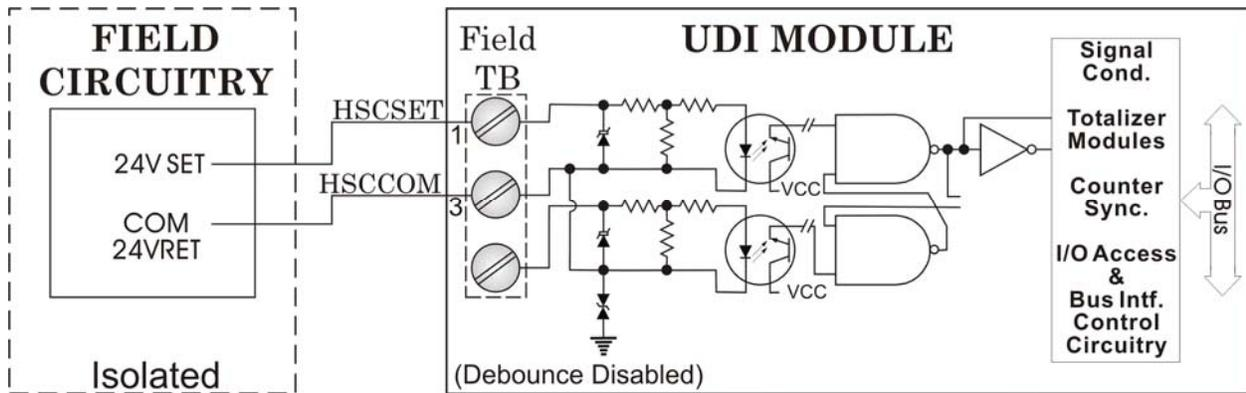
Figure 3-26. UDI (Debounce Disabled) Wiring Diagram
