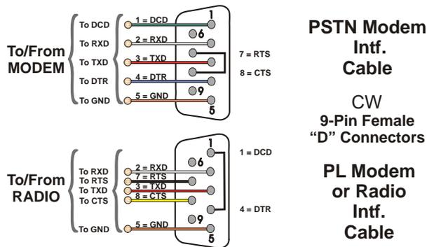
Figure 2-17. Connecting to a Modem or Radio
