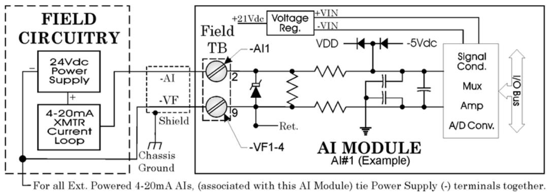
Figure 3-16. Externally Powered 4-20mA Current Loop AI - Wiring Diagram
