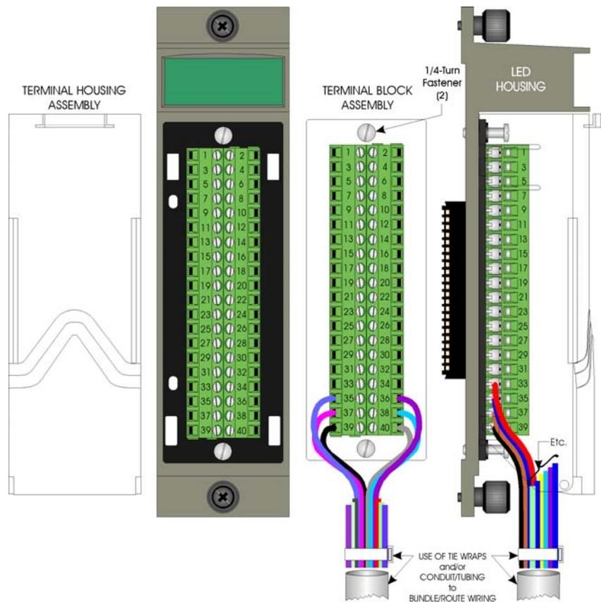
*Figure 3-3. I/O Module (Local Termination) Wire Routing*
