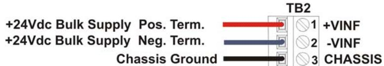
Figure 2-7. Wiring Field Power to the PSSM
