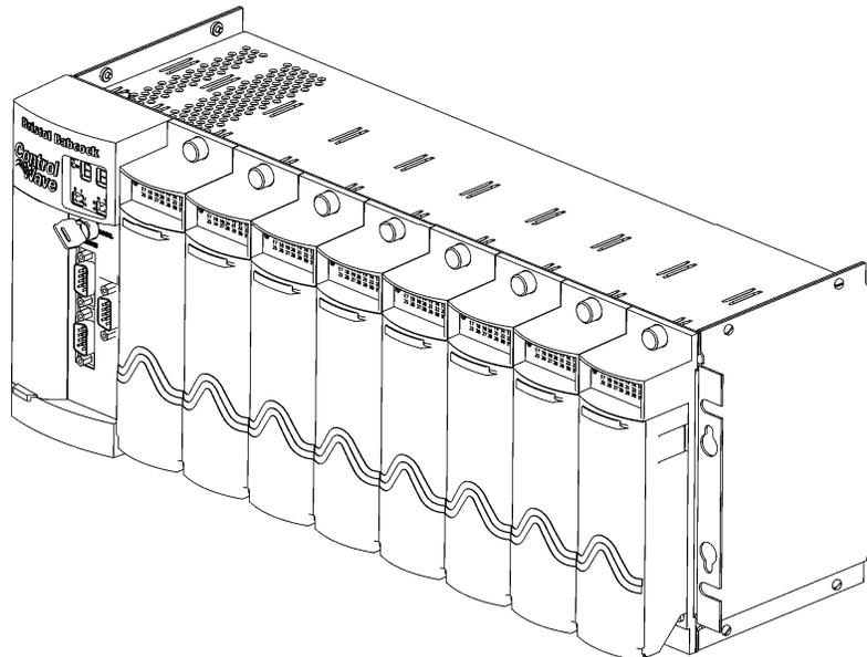
*Figure 1-1. ControlWave with 8 I/O Modules*
