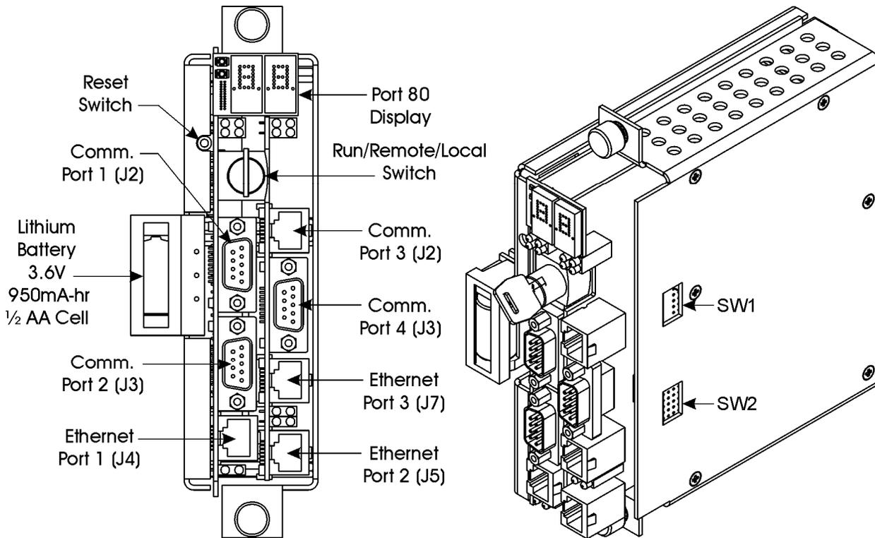
Figure 2-13. ControlWave CPU Module (with SCB)
