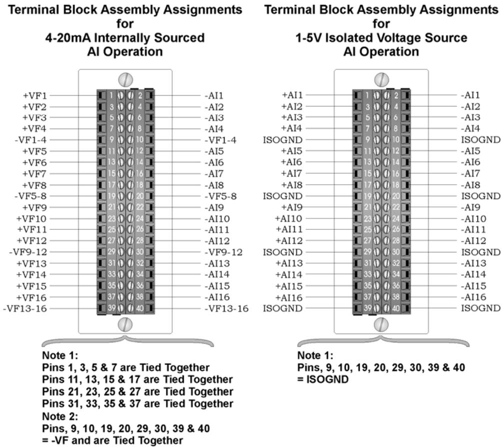
Figure 3-18. Local AI Module Terminal Blocks Assembly Assignments
