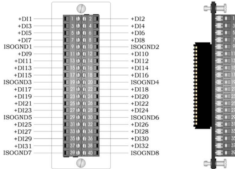
Figure 3-6. DI Module - Local Terminal Block Assembly Assignments
