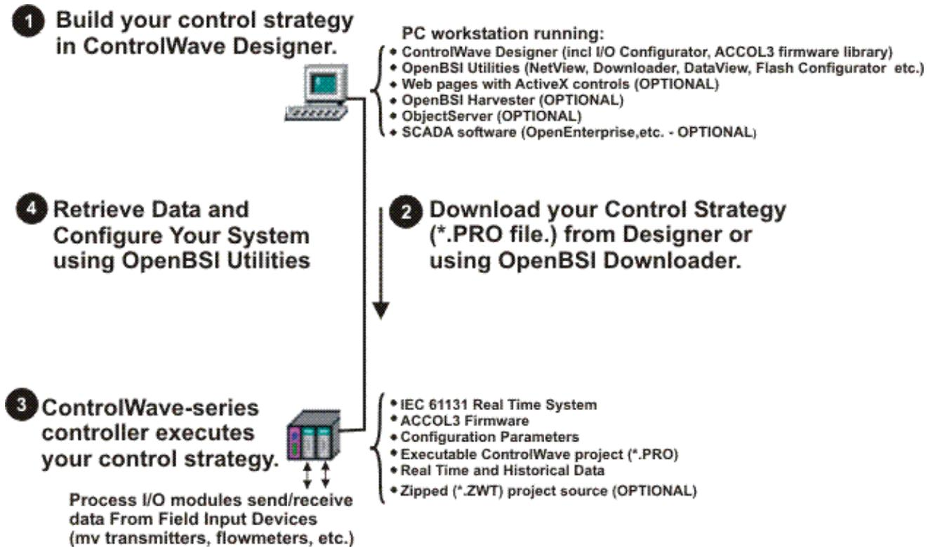
Figure 1-4. ControlWave Programming Environment
