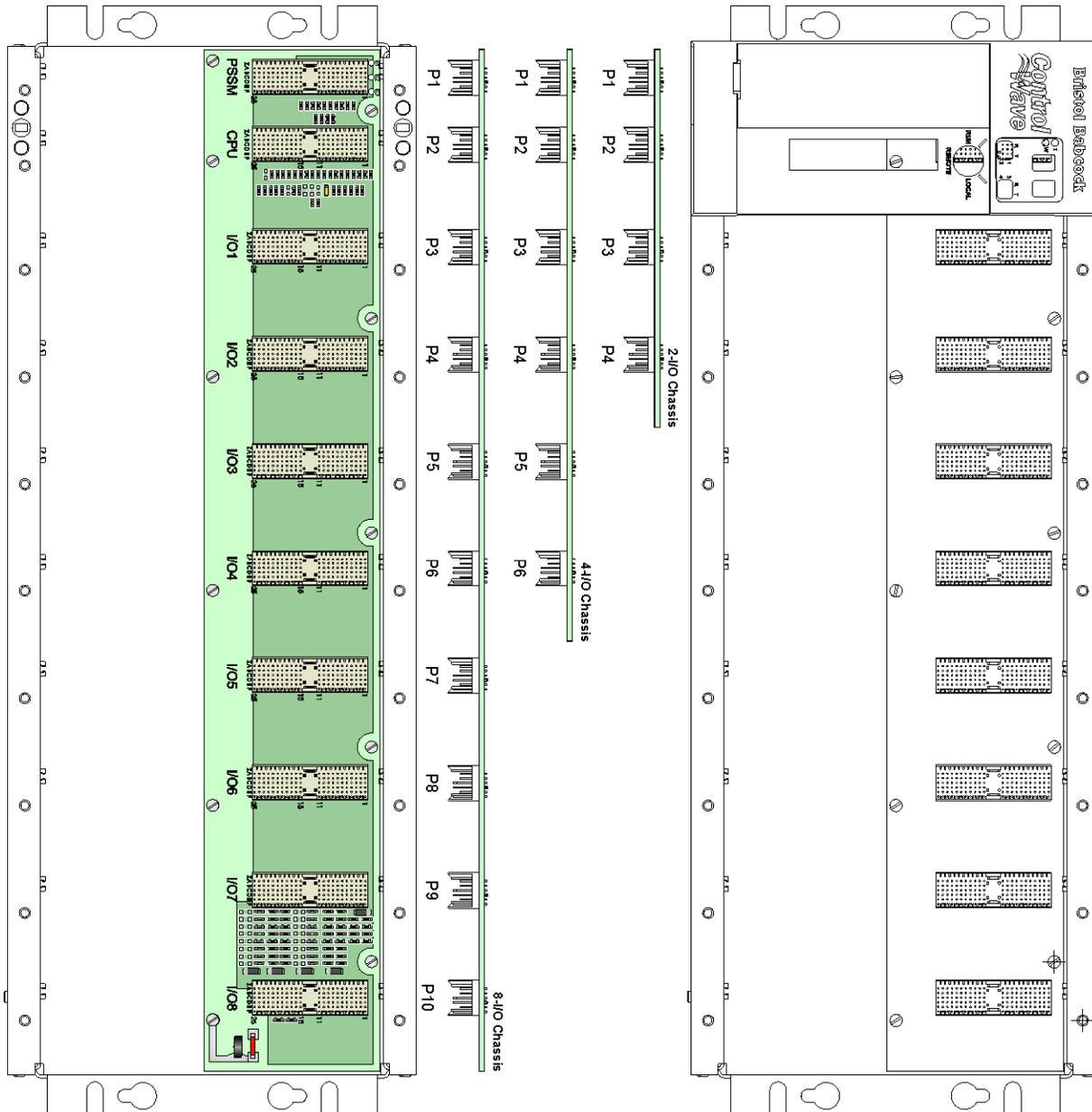
Figure 3-2. ControlWave Chassis Slot Assignments (with/without bezel shown)
