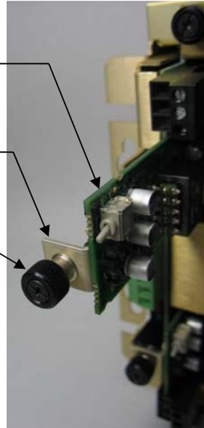
*Figure 2-8. Hot Swapping a Power Supply*
