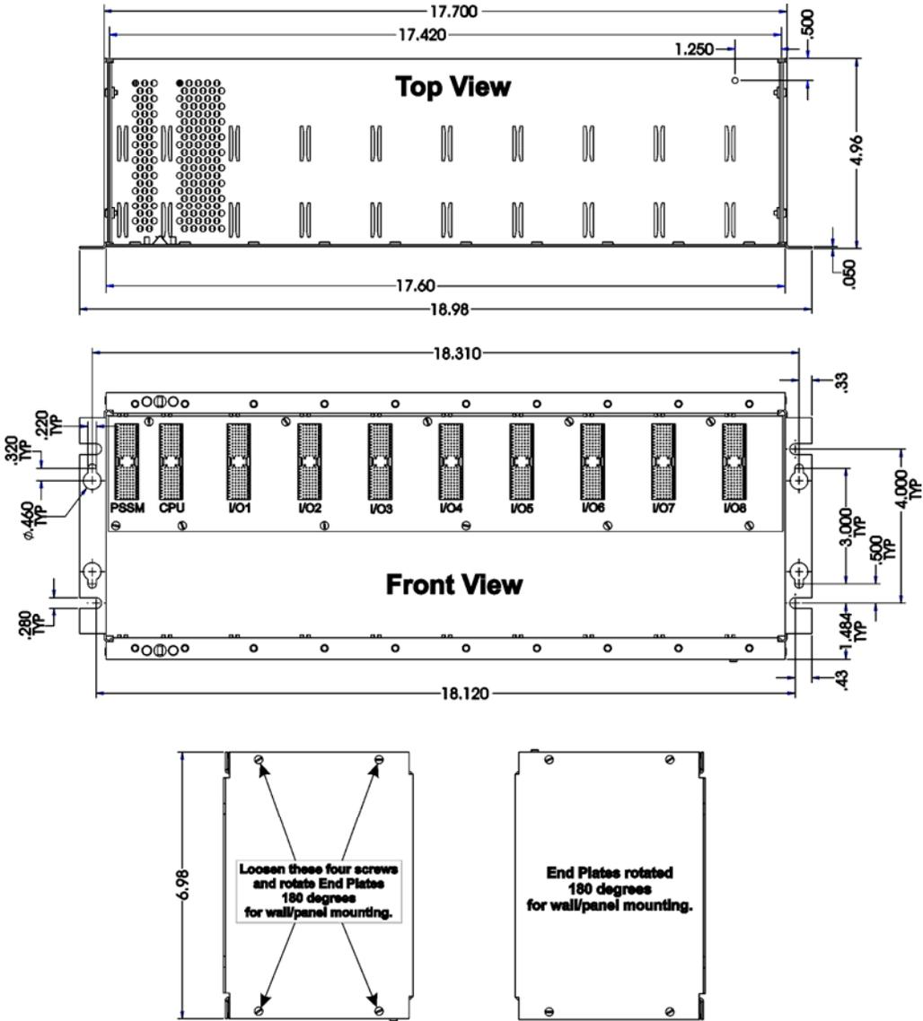
Figure 2-1. 8-I/O Module ControlWave - Mounting Diagram
