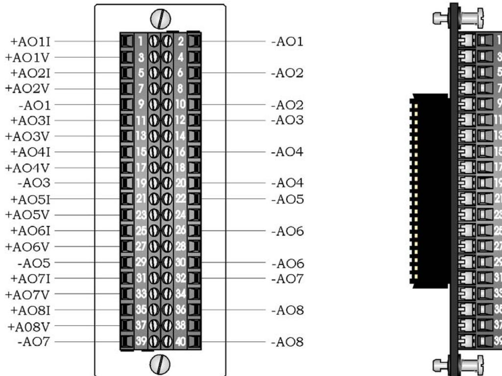
Figure 3-21. Local AO Module Terminal Blocks Assembly Assignments
