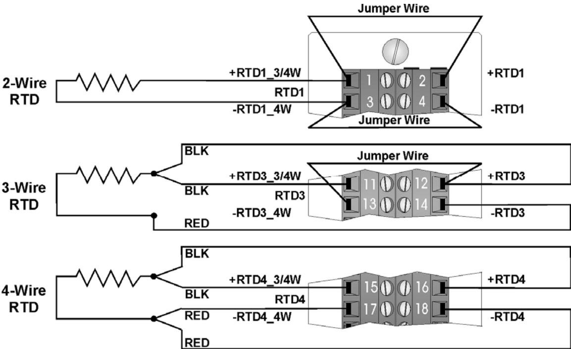
Figure 3-30. Isolated RTD Module - 2-Wire, 3-Wire & 4-Wire Wiring Diagram
