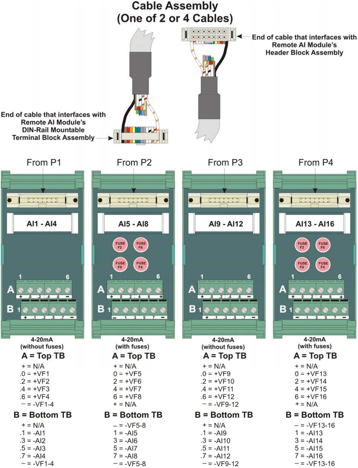
Figure 3-19. Remote DIN-Rail Mountable Terminal Block Assembly Assignments for 4-20 mA AI Operation
