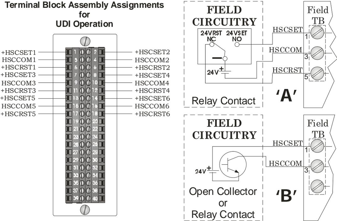
Figure 3-27. Local UDI Terminal Block/Configuration Diagram
