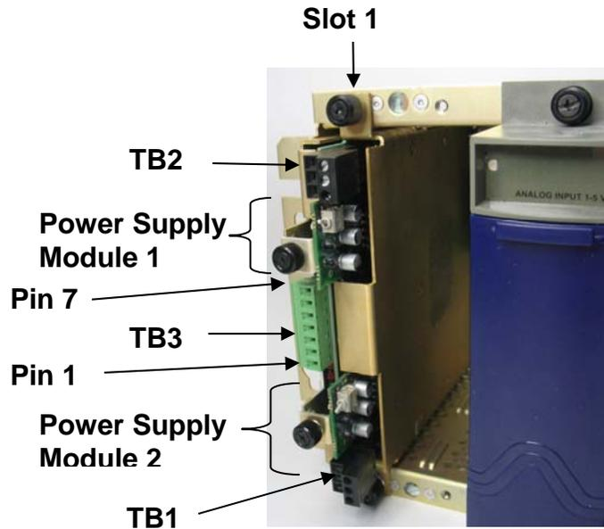
Figure 2-3. PSSM Installed in ControlWave Slot #1 of a ControlWave Controller
