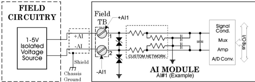
Figure 3-17. Externally Powered Isolated 1-5 Volt AI - Wiring Diagram
