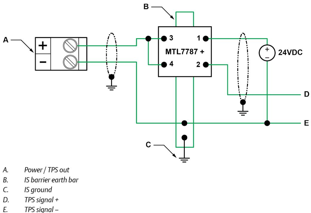
**Figure 3-3: 2-wire barrier connection with flow computer / signal converter**
