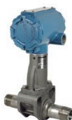
The Rosemount 8800 Threaded End Vortex flow meter simplifies installation with NPT threaded process connections which match existing threaded pipe unions.
