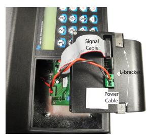
5. Disconnect the red-green power and grey signal cables from the back of the printer.
