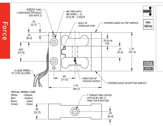
All dimensions are inches [millimeters], unless otherwise noted. Additional pin holes as shown must be used for Safe Overload on 200 lb Capacity & above.
