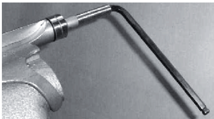
Figure 16: Bearing Removal
