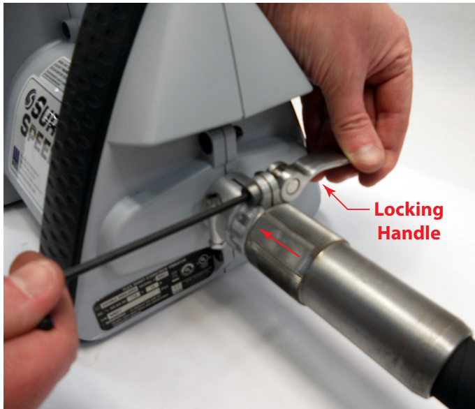
Figure 7: Locking lever adjustment
