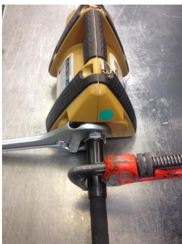
Figure 11: Crescent wrench and pipe wrench placement
