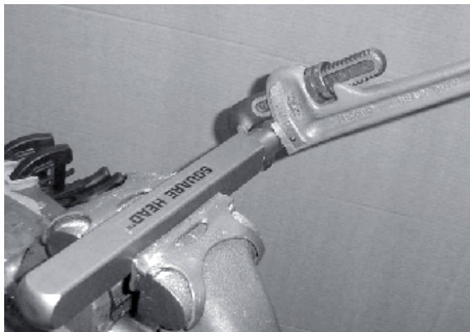
Figure 15: End cap removal
