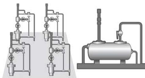
**Well Test Manager** - automation of cyclic test well separator for up to 64 wells.
