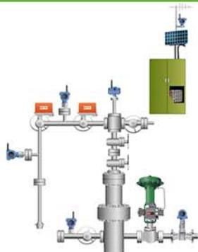
**Gas Lift for Oil** - controls and optimizes lift gas applied to oil-producing wells to maximize production.
