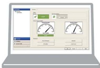
**Surface Control Manager** - allows easy configuration for balance-of-plant equipment including separators, heater treaters, shut down logic, and more.
