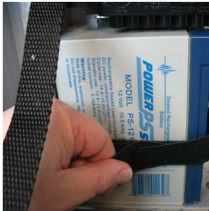
Figure 5-10: Unstrap the Old Battery Pack – Leave Connected to Cable
