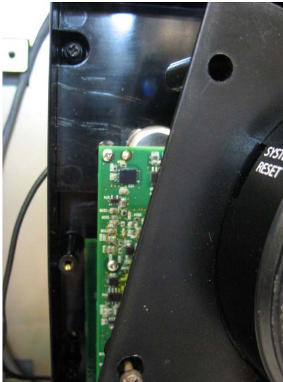
Figure 5-19: Removing the CPU Enclosure Cover
