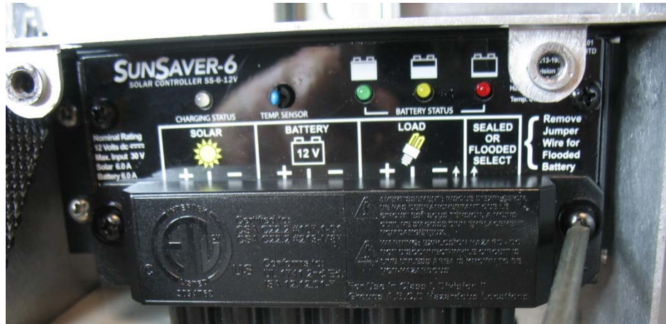
Figure 5-9: Removing the Termination Cover (if present)
