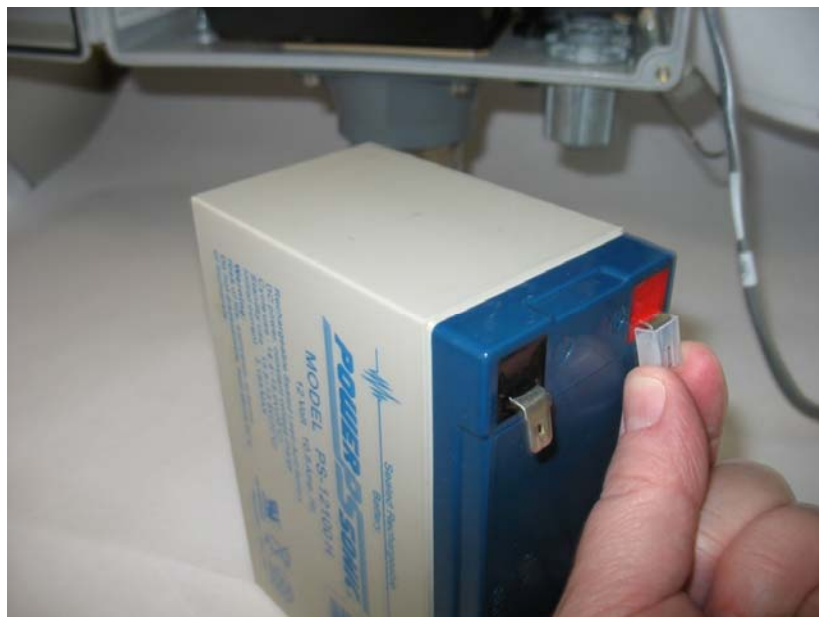
Figure 5-6: Removing Plastic Tabs from New Battery Pack
