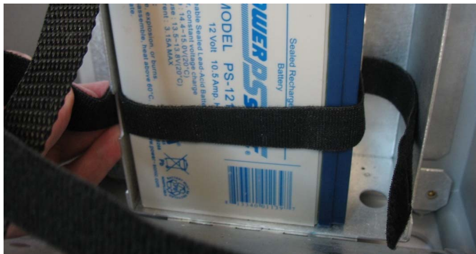
Figure 2-28: Battery Pack Attached to Compartment
