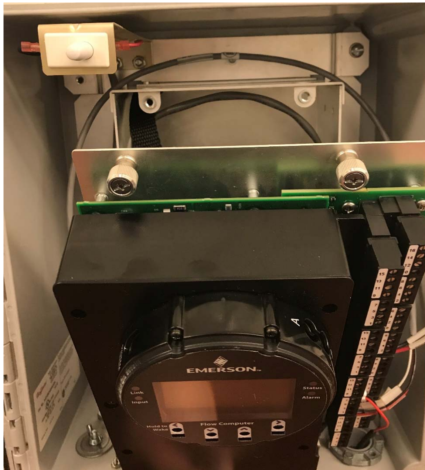
Figure 2-23: Rotate Assembly Forward
