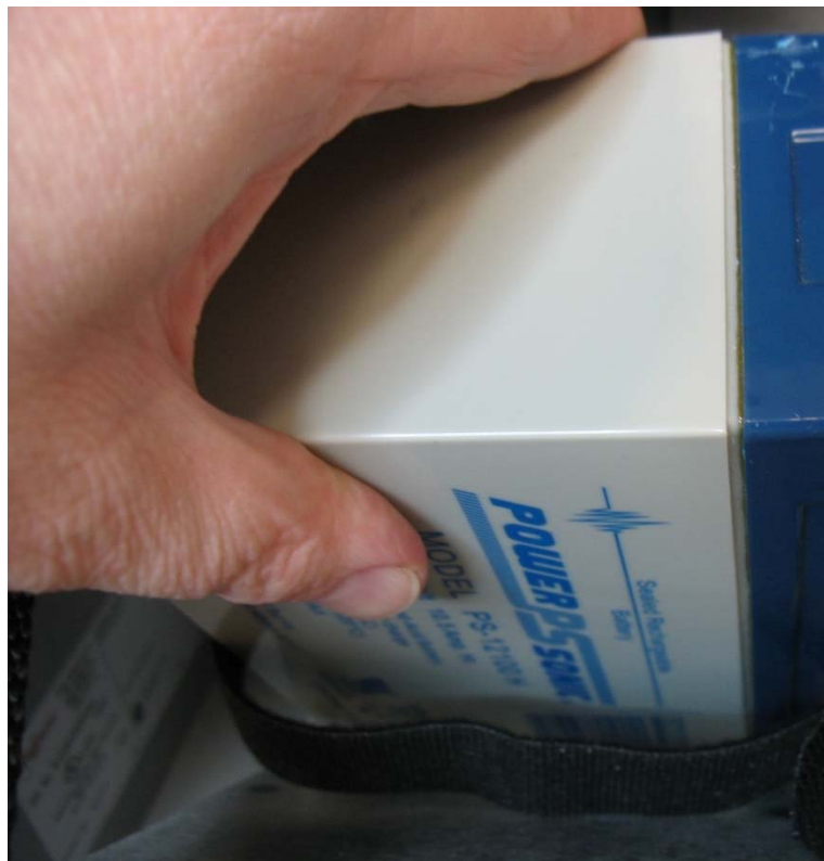
Figure 2-27: Easing Battery Pack into Compartment
