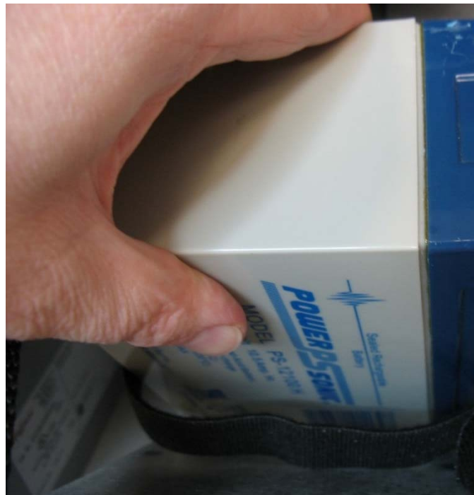
Figure 5-15: Easing the Battery into the Battery Compartment
