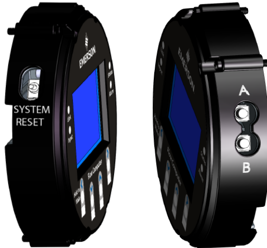
Figure 5-3: Switch and Buttons
