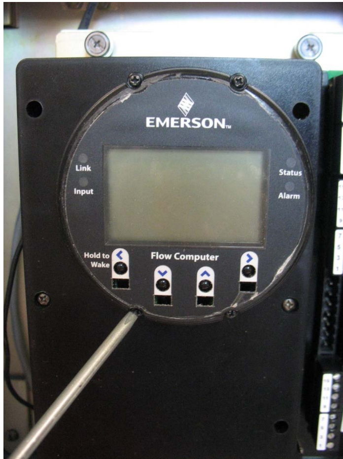
Figure 5-4: Captive Fastening Screws
