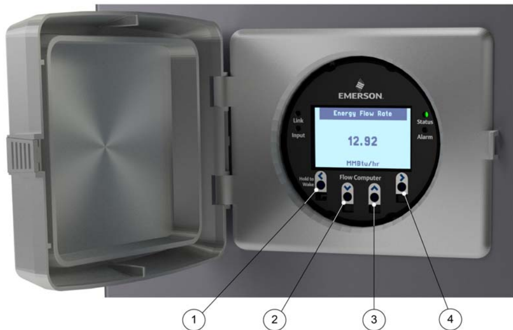
Figure 4-2: Infrared (IR) Button Location
