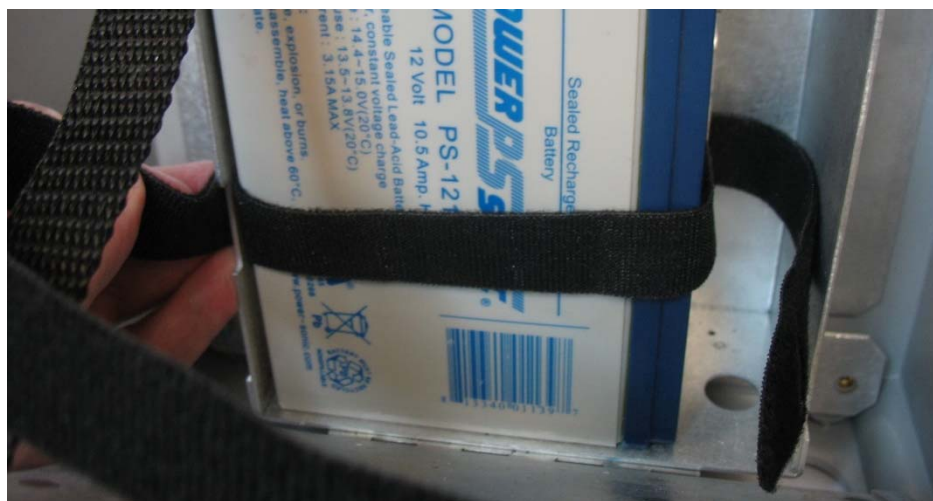
Figure 5-16: Tightening the Battery Strap
