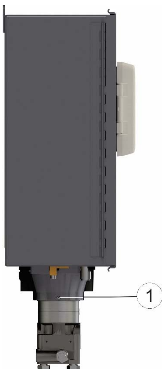
Figure 2-19: Housing Rotation Set Screw (1 each side)
