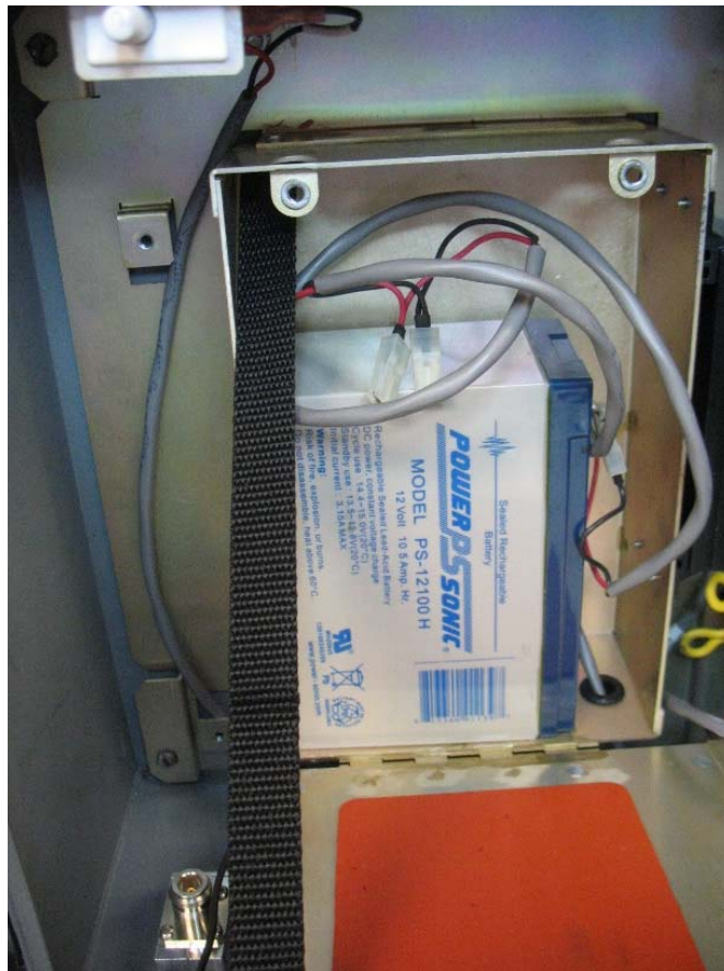
Figure 2-30: Battery Pack Attached to Compartment
