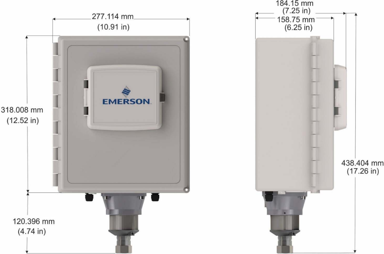
Figure 2-5: Dimensions – Static Pressure Sensor Version – Fiberglass Enclosure
