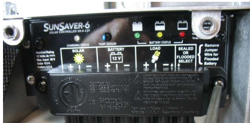
Figure 2-25: Removing Termination Cover of Internal Solar Regulator
