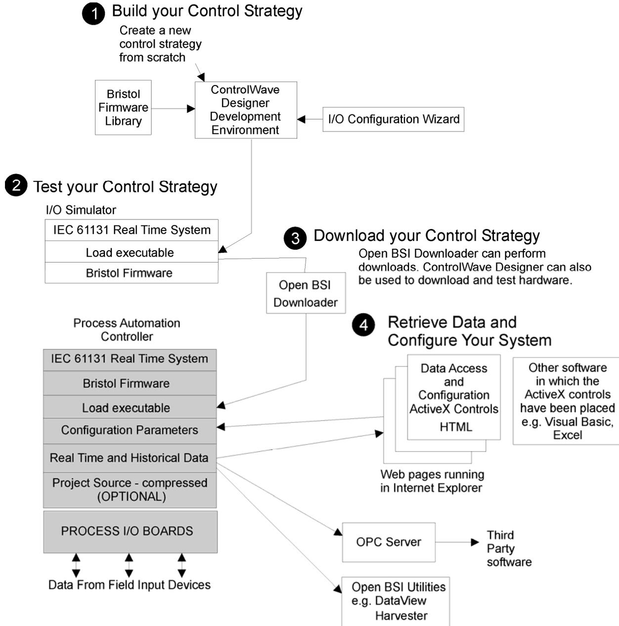
**Figure 1-2 - ControlWave - Control Strategy Software Diagram**
