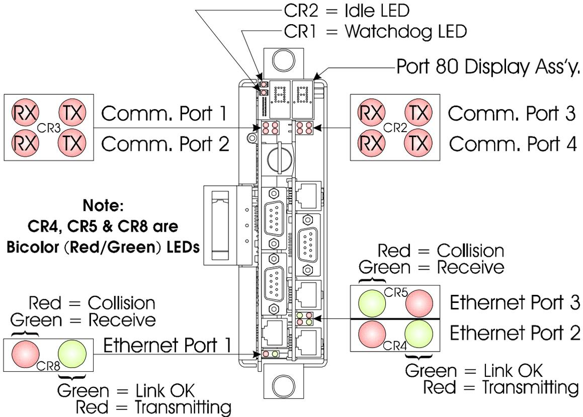
**Figure 3-5 - CPU Module Port & LED Designations**
