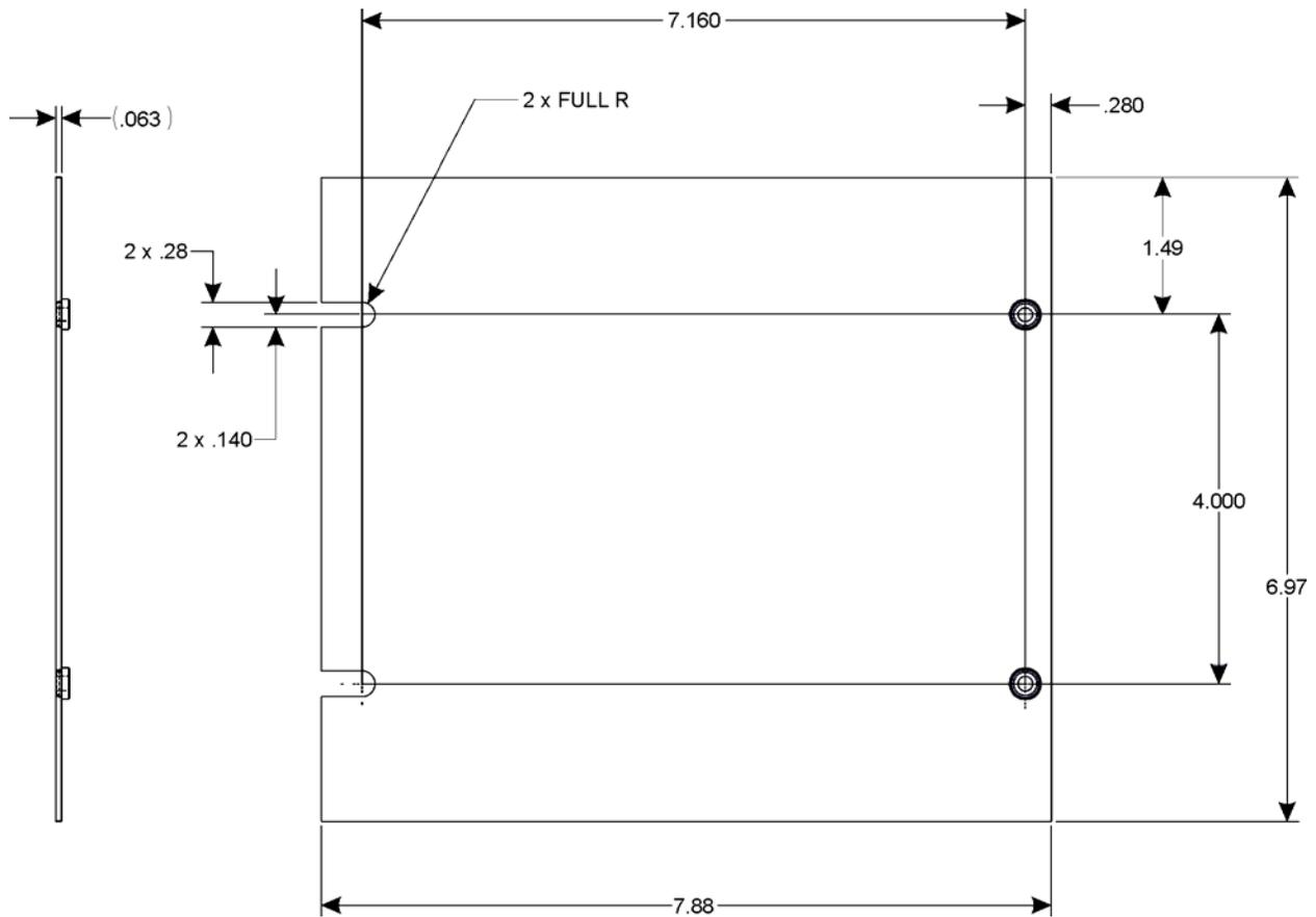
**Figure 2-2 - ControlWaveRED Rack Mount Filler Panel Dimensions**
