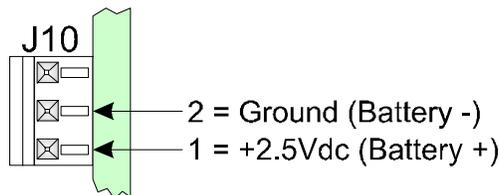
Figure 4-5 - Connector J10 - CPU Battery Header
