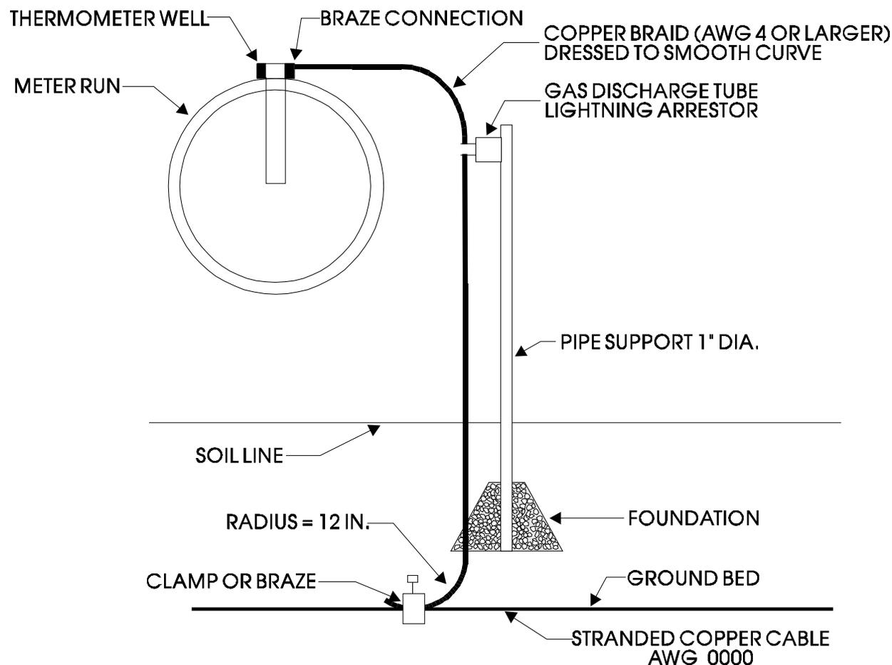
Figure 3-7 - Grounding of Thermometer Well in Gas Line
