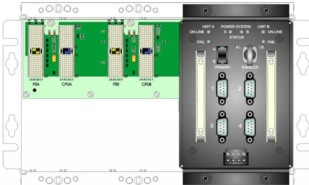
Figure 2-3 - ControlWaveRED Prior to Installation of PSSMs
