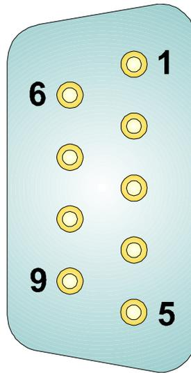
**Figure 4-2 - DB9 9-Pin Connector Port Pin Assignments**
