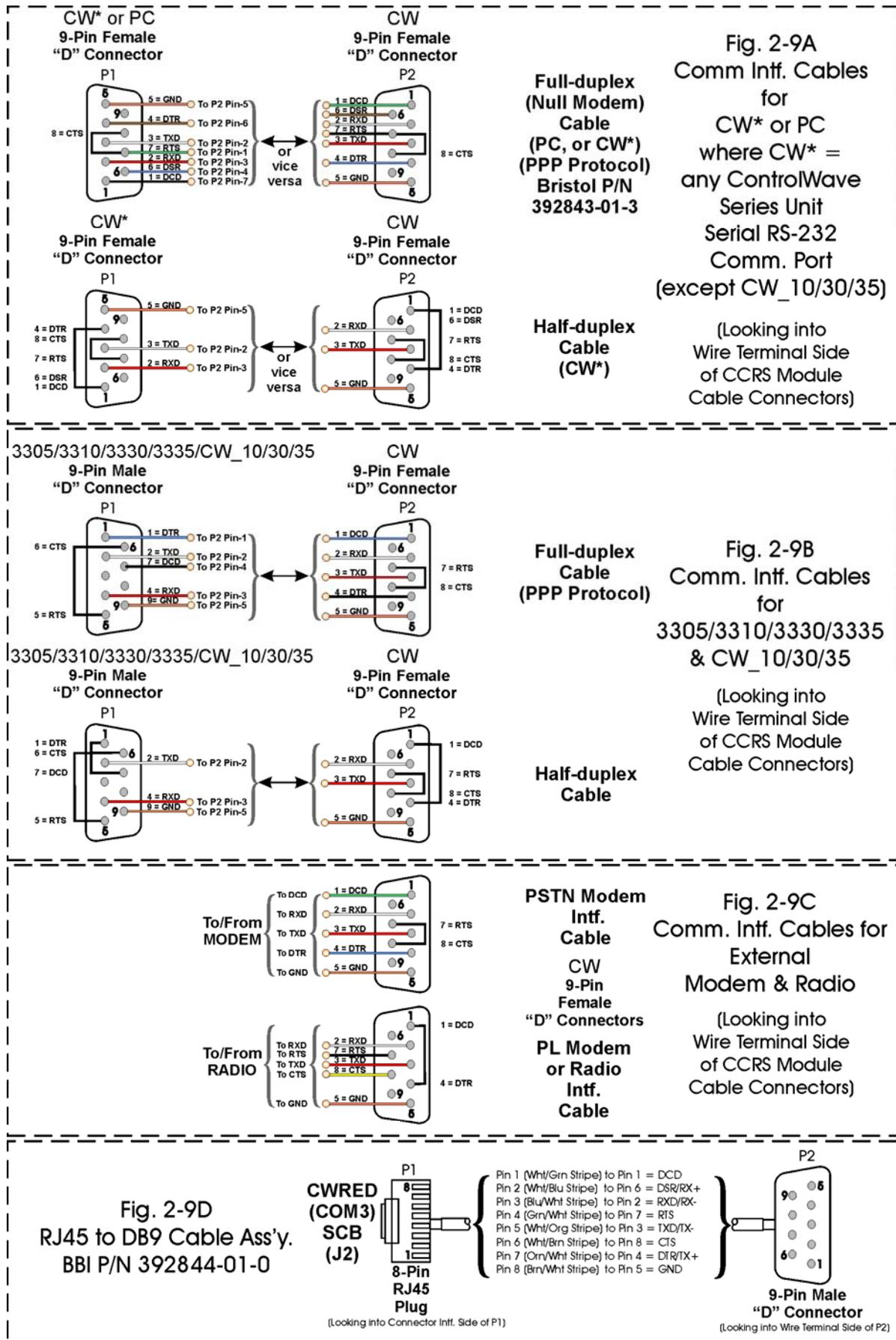
Figure 2-9 - Communication Port RS-232 Cables Wiring Diagrams
