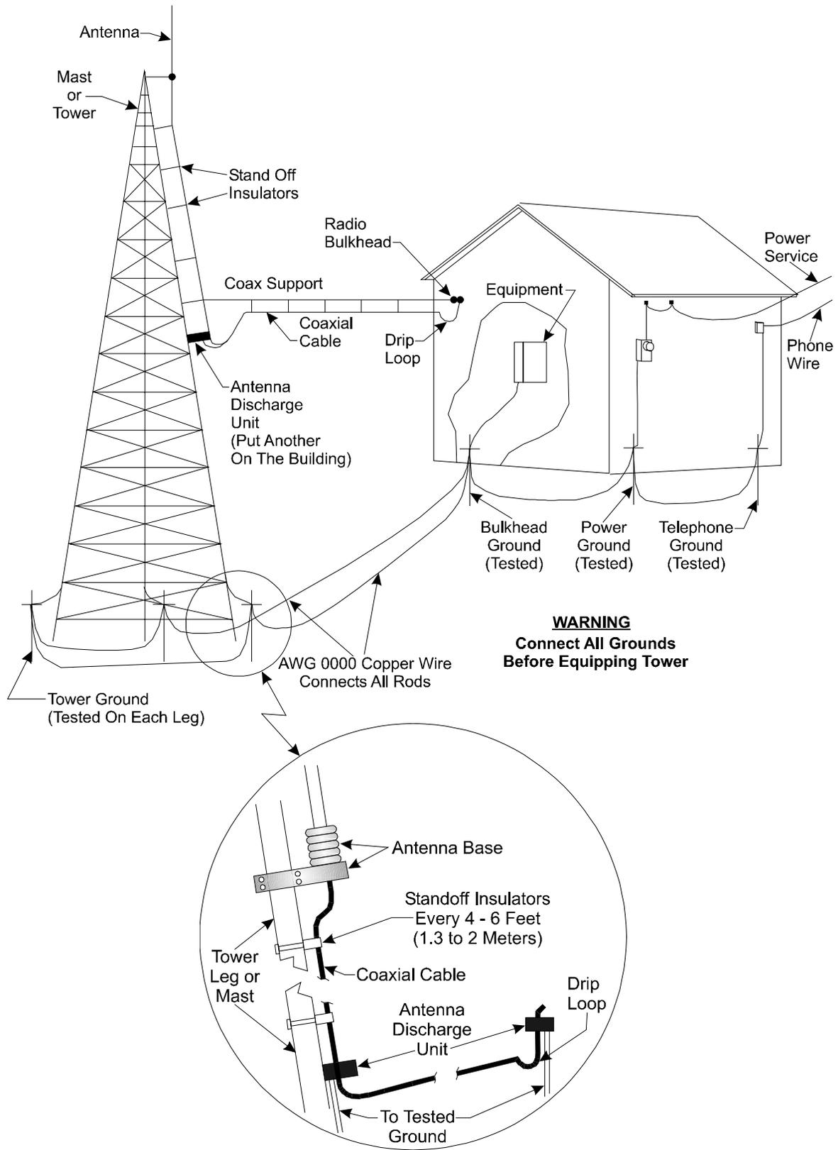
**Figure 4-2 - Radio Antenna Field Installation Site Grounding Diagram**
