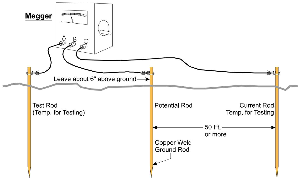
**Figure 3-2 - Basic Ground Bed Soil Test Setup**
