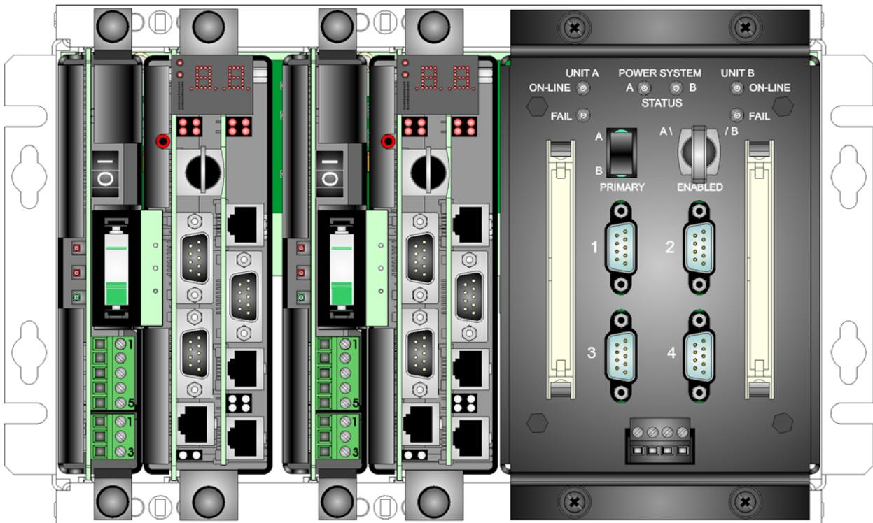
**Figure 2-5 - PSSMs & CPUMs Installed in ControlWaveRED Slots #1 through #4**
