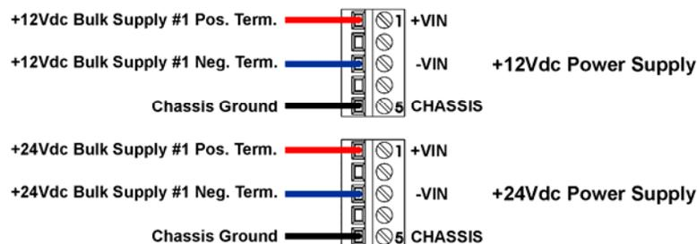
**Figure 2-16 - PSSM TB2 Typical Wiring Schemes**
