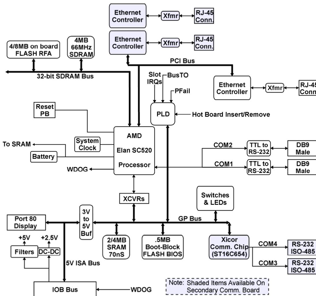
Figure 1-3 - Block Diagram of ControlWave™ CPU Board
