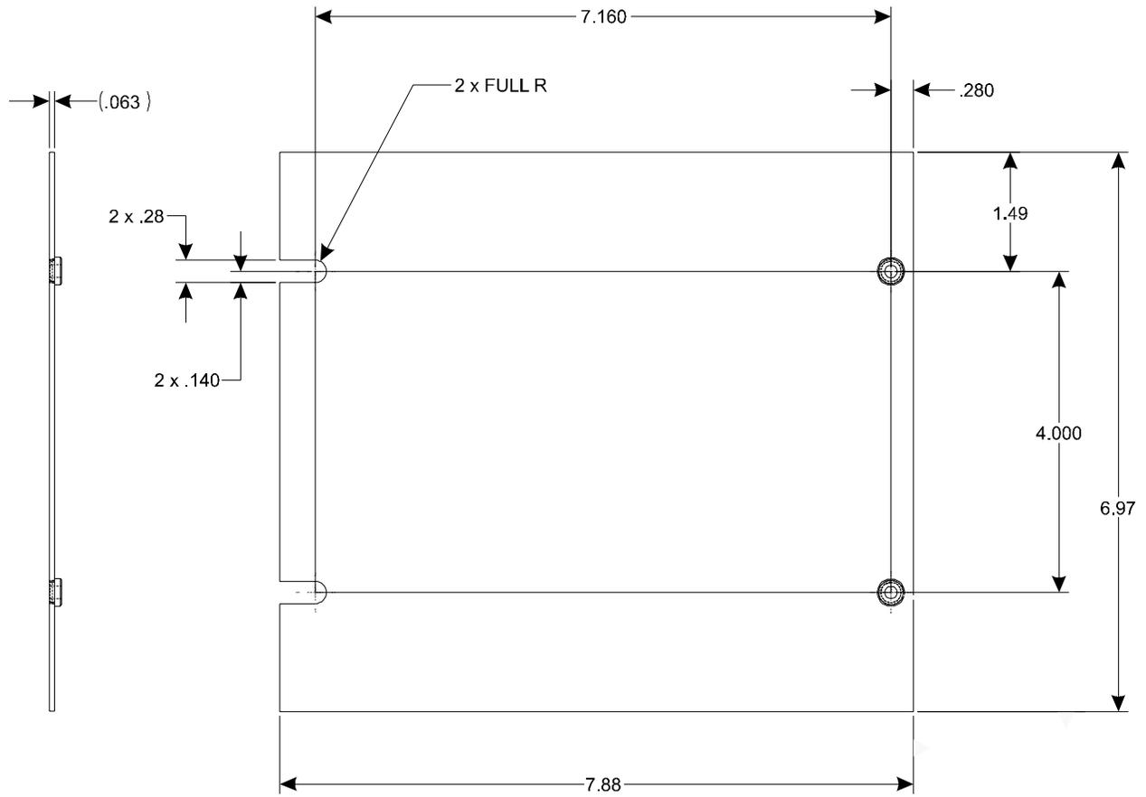
**Figure 4-10 - ControlWaveRED Rack Mount Filler Panel Dimensions**
