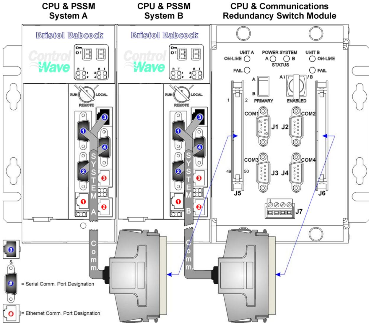
**Figure 2-8 - Redundant Communication Cables Connection Diagram**
