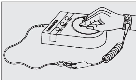
**Note:** If a system checker is not available, use an ohmmeter connected to the cable ends to measure its resistance. The ohmmeter reading should be **1 megohm +/- 15%**. Be sure that the calibration date of the ohmmeter has not expired. If the ohmmeter reading exceeds **1 megohm by +/- 15%**, replace the ground cord with a new one.
