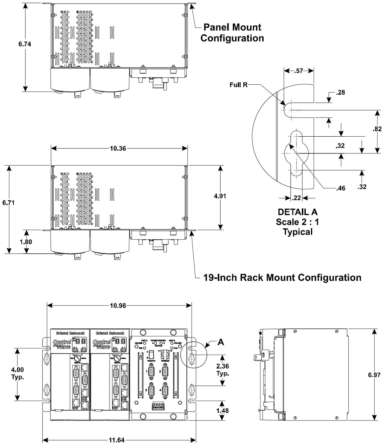
**Figure 4-9 - ControlWaveRED Dimension & Installation Drawing**
