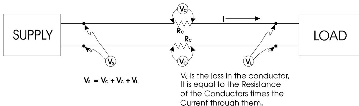
**Figure 5-2 - Calculating Load Voltage due to Line Resistance**
