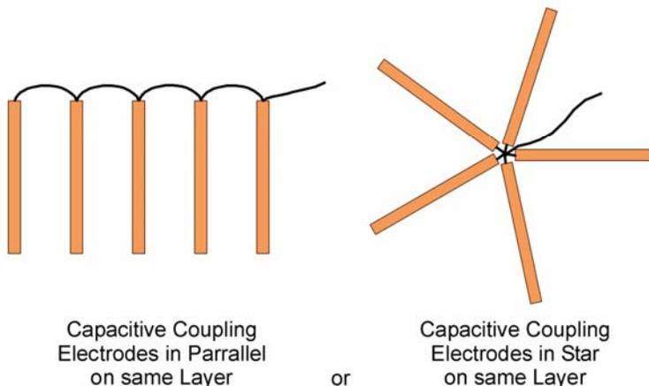
**Figure 3-5 - Poor Soil Ground Bed Construction Diagram**
