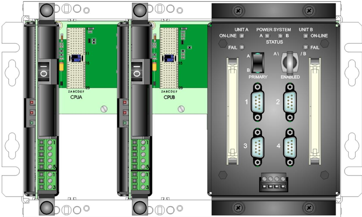
**Figure 2-4 - PSSMs Installed in ControlWaveRED Slots #1 and #3**
