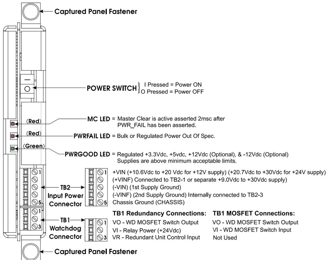
**Figure 3-4 - Power Supply/Sequencer Module's TB1, TB2 & LED Designations**
