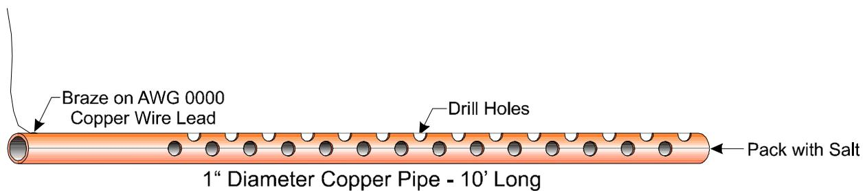
**Figure 3-4 - Ground Electrode Construction for Poor Soil Conditions**
