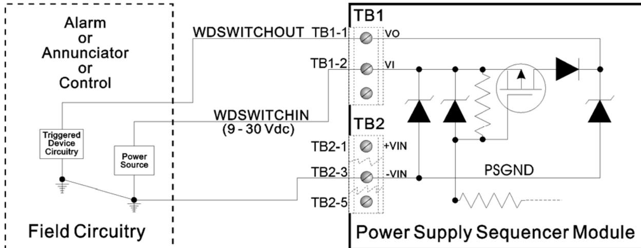
Figure 2-17 - Watchdog MOSFET Switch Field Wiring
