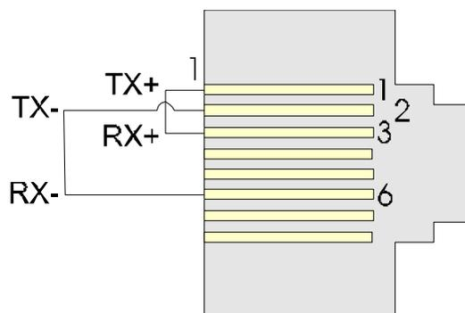
Figure 3-12 - RJ-45 Ethernet Loop-back Plug
