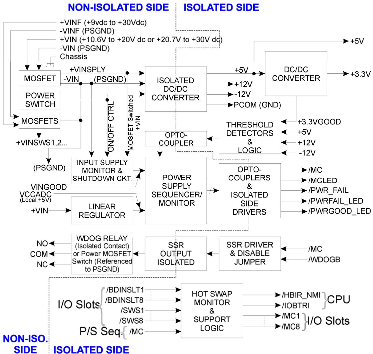
Figure 1-7 - Power Supply/Sequencer Module Block Diagram
