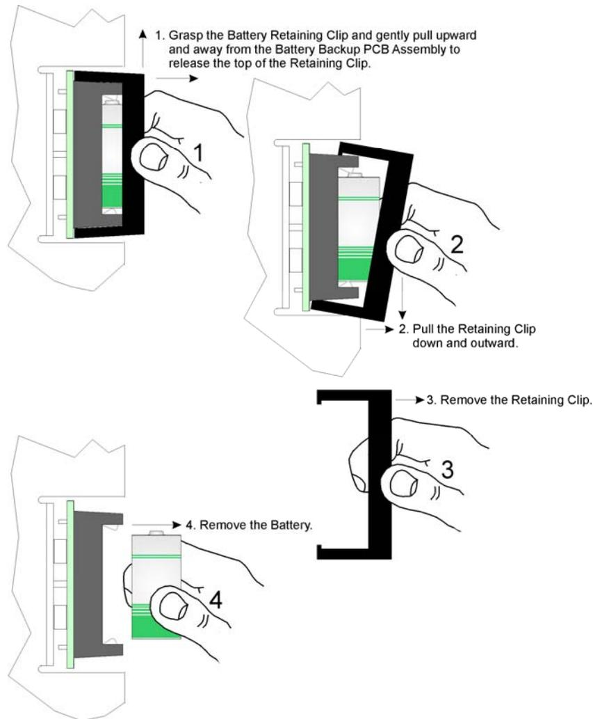
**Figure 2-19 - Lithium Backup Battery Removal Diagram**
