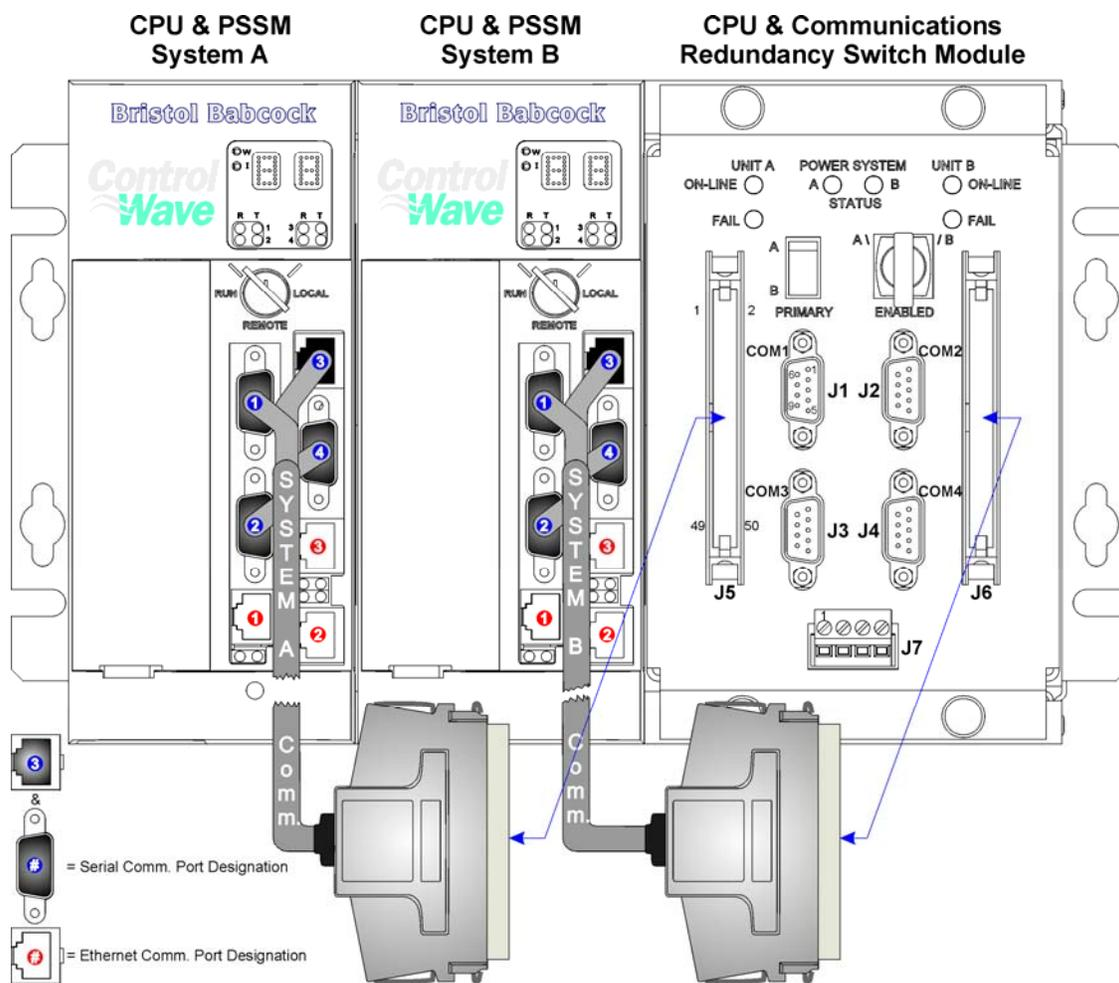
**Figure 1-12 - ControlWaveRED Chassis and Comm. Cabling Diagram**
