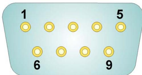
**Figure 2-10 - Male DB9 9-Pin Connector (CPUM: COM1, COM2 & COM4)
