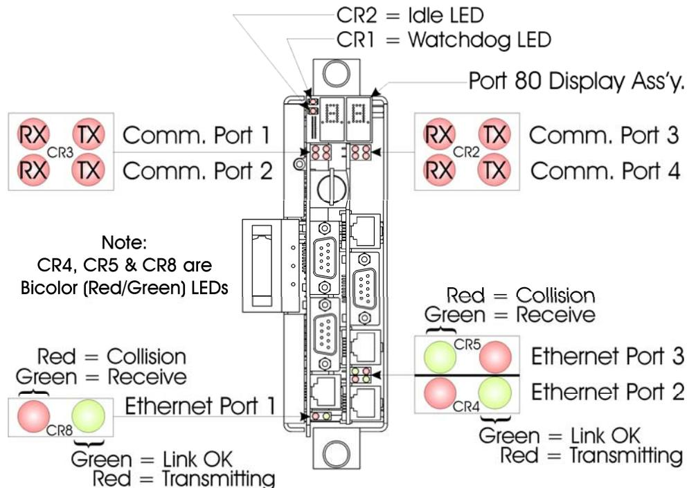
Figure 1-5 - CPU Module LEDs
