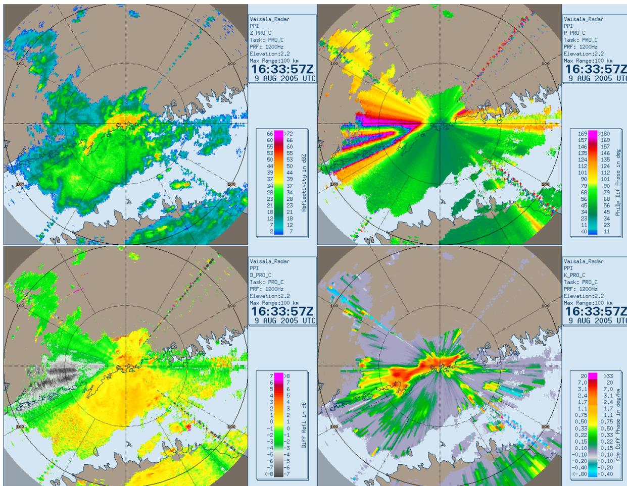
Fig. 2. Example of sweep data acquired by the Kumpula weather radar in event of intense convection. Top left: the field of reflectivity, top right: field of differential phase, bottom left: field of differential reflectivity, bottom right: field of specific differential phase computed with the adaptive  $K_{dp}$  method (adaptive scaling factor 0.5).
