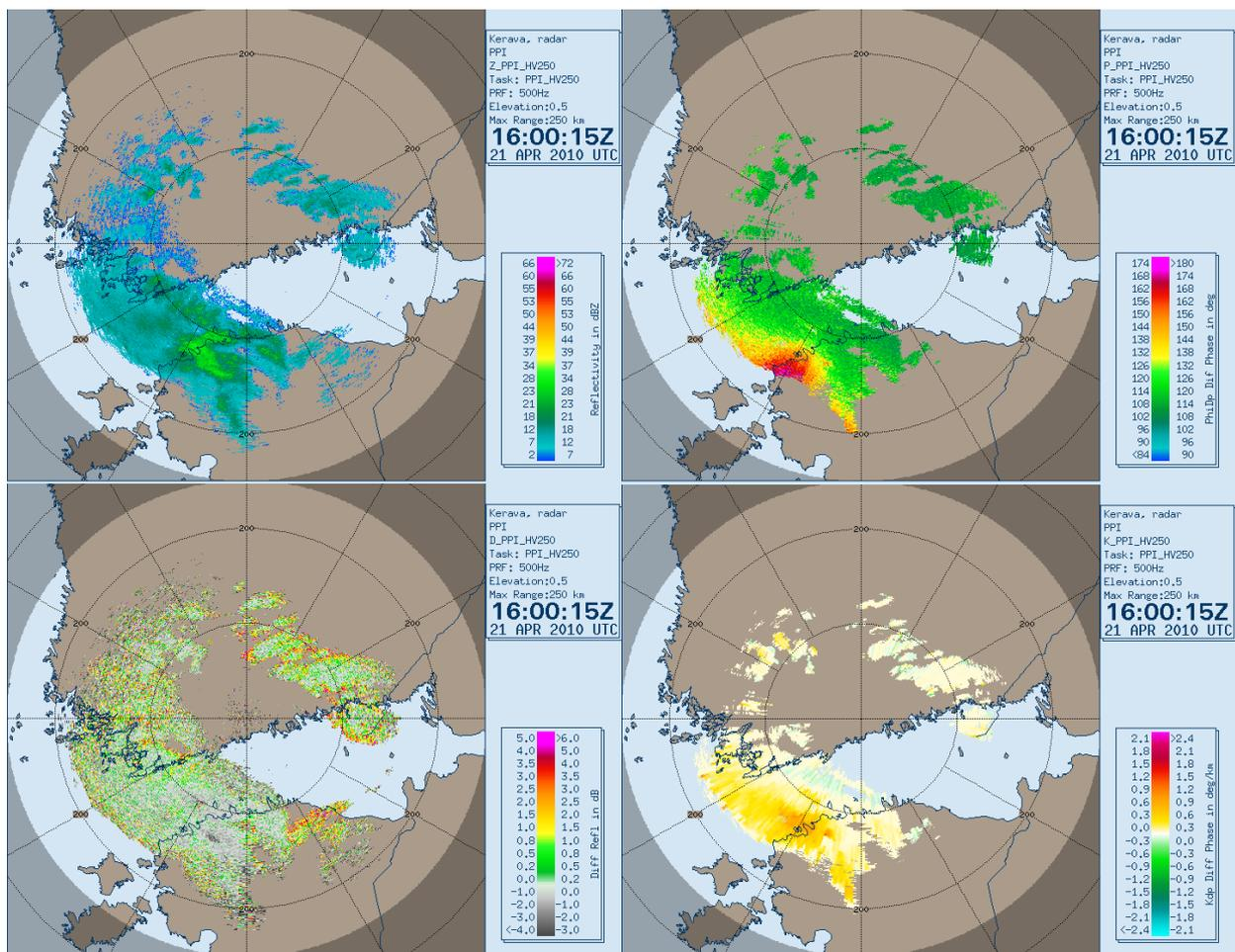
Fig.1. Example of sweep data acquired by the Kerava WRM200 radar in large scale precipitation. All moments are Doppler filtered for ground clutter. Top left: the field of reflectivity, top right: field of differential phase, bottom left: field of differential reflectivity, bottom right: field of specific differential phase computed with the adaptive  $K_{dp}$  method (adaptive scaling factor 0.5).
